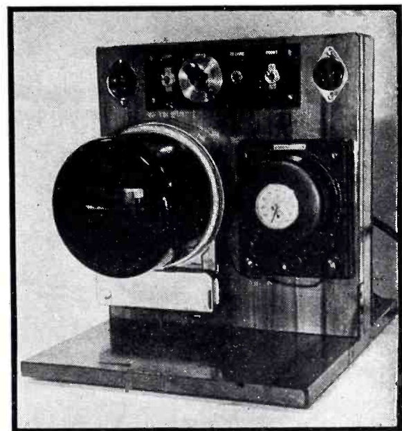
FIG. 3—Schematic diagram of light actuated impulse counter, used with small wattmeter to record total amount of energy for heating the test boxes
