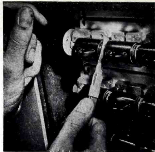
Method of checking spark gap with a feeler gauge and adjusting gap thickness with a wrench. The loops of copper tubing carry cooling water between holes drilled transversely through the brass cylinders which support the tungsten electrodes
