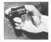
tivity, control characteristics practically independent of ambient temperature over a wide range, relatively unaffected by line-voltage surges, maximum peak inverse anode voltage rating of 1300 volts, instantaneous current rating of 500 ma. and an average current rating of 100 ma. The quick-heating cathode is rated at 6.3 volts, 0.6 amp.
