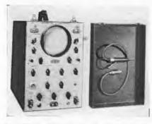
Mc. The X-axis or horizontal deflection amplifier has a uniform characteristic from 10 cps to 100 ke. Both amplifiers have distortionless input attenuators and gain controls. Provision is made to connect signals directly with the deflection plates when frequencies to be observed are beyond the useful limits of the amplifiers.
