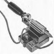
This is a thermostatically controlled device for the regulation of the temperature of an electric soldering iron. When placed on and connected to this stand, iron may be maintained at working temperature or through adjustment on bottom of stand at low or warm temperatures.
