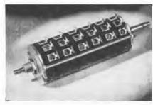
locks with each rotor in the stack. Thus the finished assembly is really a single control with several independent sections for as many independent circuits. All units pass through the same degree of rotation as the single shaft is rotated. Individual units can be of any standard resistance, taper, taps and hop-offs to meet individaul circuit requirements.
