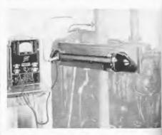
Fig. 1-Combustion efficiency of this diesel engine is indicated in terms of exhaust smoke density when a suction fan pulls part of the exhaust gas through a beam of light in an 18-inch tube mounted on the engine
