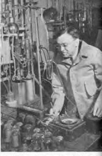
Dr. Harvey C. Rentschler conducting a experiment in which oxygen gas is being dissolved in a strip of zirconium meta enclosed in the glass tube suspended directly in front of him
