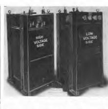
The unit is also light and compact and requires no headroom. It is constructed throughout with class B. heatproof insulation consisting of fiber glass, mica, asbestos and porcelain. The trausformers are available up to 500 kva; in voltages to 4800 volts, single phase, three phase, and Scott connected 3 to 2, or 2 to 3 phase, in one unit.
