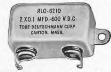
CHARACTERISTICS - TOBE RLO TYPE CAPACITORS MINERAL OIL IMPRESNATED -- Mineral oil filled + RATINGS: .01 to 2.0 mfd., 600 V.D.C., .01 to 1.0 mfd., 1,000 V.D.C. POWER FACTOR: At 1,000 cycles -. 002 to .005 . RESIS-TANCE: 8,000 megohms per microfarad . TEST VOLTAGE: Twice D.C. working voltage rating . TERMINALS TO CASE TEST: 2,500 Volts D.C. . STANDARD CAPACITY TOLERANCE: plus or minus 20% of nominal
