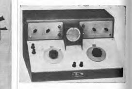
of rugged design are included oscillator and amplifier circuits are permeability tuned and have silver-mica condensers to minimize frequency and phase shift: visual method of indication reduces operator fatigue; only fixtures and jigs are required for connecting different coils to the test terminals; and finally, various parts of the unit are readily available for periodical inspection. Radex Corp., 1733 Milwaukee Ave.,
