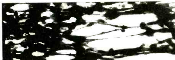
Micrograph showing Vinylite in one of its many stages of polymerization. The study of plastics is aided by the RCA Electron Microscope, which enables observation of the polymerization process, typical of the plastics.
