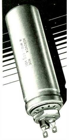
Something new has been added to this long-popular Aerovox "10" series Hyvol capacitor. Note the double terminals spaced on the stepped bakelite threaded terminal post. This means the can of this handy inverted-screw-mounting capacitor is now insulated or "floating". No longer is an insulator washer required when non-grounded mounting on a metal chassis is desired.
