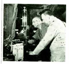
GE's Dr. Saul Dushman adjusts a wire sample while J. T. Mireles Malpica, who substituted a phototube for an eye at a microscope as a means of measuring "creep" rate, looks on
