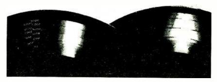
Fig. 3—Light-patterns on two frequency records made by the same cutter, the one at the left through the single-ended amplifier discussed in the text and the one at the right through a commercial push-pull amplifier without feedback
