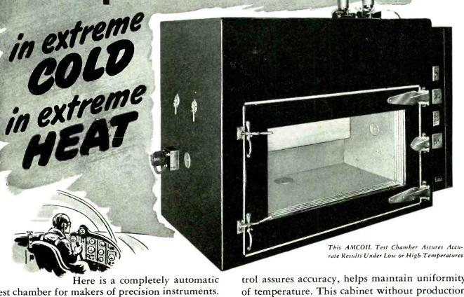
Here is a completely automatic test chamber for makers of precision instruments. Here is a way to give delicate mechanisms scientifically-created "previews" of performance conditions. The Amcoil Model RTC-1 is an all-steel test chamber combining mechanical refrigeration and electric heating.
