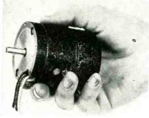
housing is 2.306 ins; overall length, not including the shaft extension, is 215 ins; it weighs 1 lb and 3 oz; the shaft diameter is 0.250 ins; the shaft extension is 0.766 ins. The motor is equipped with ball bearings and is reversible (3 leads)
