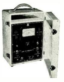
accurate to one-tenth of one percent and the indicating meter is a 42-inch galvanometer having a sensitivity of 25-0-25 microamps.
