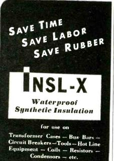
Solve your wartime insulation problems with INSL-X, the improved waterproof synthetic insulation. Today, when every penny, every minute, every it's time to turn to INSL-X for extra economy, new ease of application, improved all-around insulation efficiency. Easy to apply by brush, dip, or spray -INSL-X gives initial dielectric strength of 1500 volts per mil. which increases rapidly with aging.
