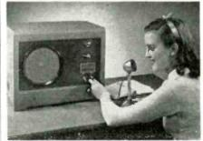
A new Western Electric magnetic recording device is now being used by many as an aid to speech improvement. The subject's speech is recorded magnetically on a steel tape. By turning the switch immediate playback is possible, which enables the detection and correction of errors of pronounciation, emphasis, or tone. As it records, the mirrophone automatically erases or demagnetizes previous recordings
