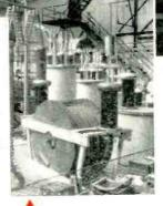
RECOVERING VALUABLE PARTICLES from flue gases in smelters, sulphuric-acid plants, cement mills, plants for de-tarring natural gases, etc. In many applications, as in the fly-ash precipitator above, pre-cipitators powered by keno-trons are used to remove solid particles from factory smoke which would otherwise be de-posited over the surrounding country. PARTICLES from flue gases in
