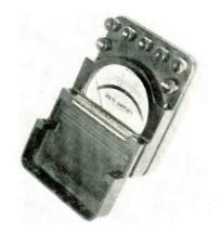
accurate readings. P-14 embodies a variety of single, and multi-ranges providing for the measurement of a-c volts, amps and milliamps: d-c volts, amps, milliamps, and micro-amps. Ranges and combinations of ranges have been chosen to meet the needs of test men, laboratory technicians and research engineers. Combinations of four current and three voltage ranges are available. The molded cases are fully insulated and magnetically shielded from stray field influence.
