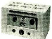
RIDENOUR - LAMPSON IONIZATION GAUGE FOR MEASUREMENT OF PRES-SURES IN REGION OF 10<sup>-4</sup> TO 10<sup>-7</sup> MM MERCURY
