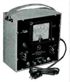
operation through appropriate terminal connections and a throw-over supply switch. Readings are made quickly and easily. The instrument is equipped with a  $4\frac{1}{2}$ -inch rectangular meter having a movement of 0-200 microamps. Ranges are 0-3-6-30-150 volts. Tubes used are type 6K6GT, 6X5GT, 6H6 and VR105-30. The latter is a voltage regulator, eliminating errors due to line voltage fluctuations.
