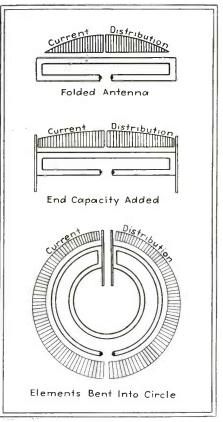
Fig. 11—Diagrams illustrating the development of the circular antenna from the folded doublet, at top
