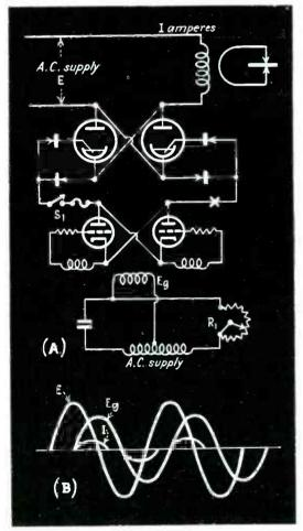
FIG. 3—(A) Contactor with simple phase control added. The amount of current passed to the welding machine depends upon the position of  $R_1$ . (B) Phase relations of line voltage  $E_r$  grid voltage  $E_p$  and line current I for one position of  $R_1$ .
