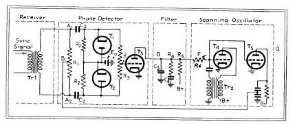
Fig. 7—Schematic diagram of connections of the phase detector and scanning oscillator of the AFPC television circuit
