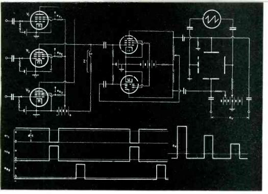
Fig. 15—By applying various input voltages to the grids of the amplifier tubes  $V_{1\nu}$   $V_{2\nu}$  and  $V_{3\nu}$ , these voltages may be combined and the resultant effect viewed on the screen of the cathode-ray tube
