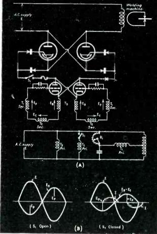
FIG. 4-(A) Another form of phase control, added to an electronic contactor. The amount of current that will flow to the welder is determined by the position of  $R_1$  (B) Voltage and phase relationships, as explained in the text
