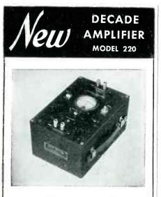
A highly stable amplifier giving gains of exactly 10 and 100 times. Operated by self-contained batteries. Through the use of special circuits the gain is independent of battery voltage, circuit constants and tubes within 2% from 10 to 100,000 cycles. Particularly useful with our Model 300 Electronic Voltmeter to increase its sensitivity, permitting voltage measurements down to 30 microvolts. Send for Bulletin 7.
