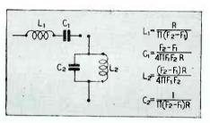
Fig. 1—Constant K band pass filter circuit
