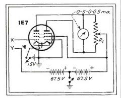
Fig. 2—Circuit for measuring resistance of moisture film condensed on inside of glass jacket
