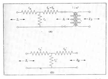
Fig. 1—Symmetrical T pad and ideal transformer (A) and the electrically equivalent dissymmetrical T pad (B), both having the same loss
