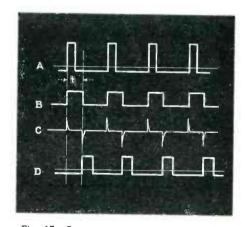
Fig. 17—A square-wave generator rather than the transmission line may be used to provide suitable time delays
