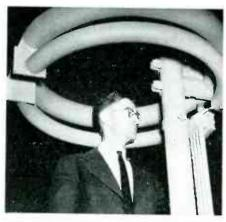
The circular antenna, described by M. W. Scheldorf, has unusual applications for use on vehicles, because of its ruggedness and small size
