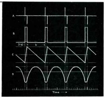
Fig. 14—Derivative and integral waveforms frequently encountered. Any one waveform is the derivative of the waveform immediately below it; conversely it is the integral of the waveform immediately above it
