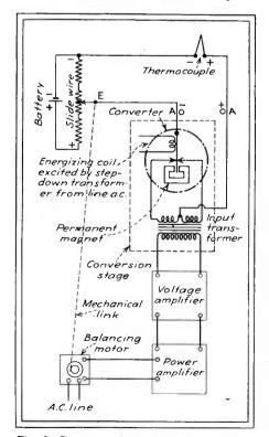
Fig. 1—Diagram of the complete continuous balance potentiometer pyrometer system
