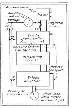
Fig. 1—Block diagram of the electronic profilometer, showing diamond-point p.m. pickup tracer head, amplifier with inverse feedback, velocity compensating integrating circuit, rms microinch meter and provision for calibration check
