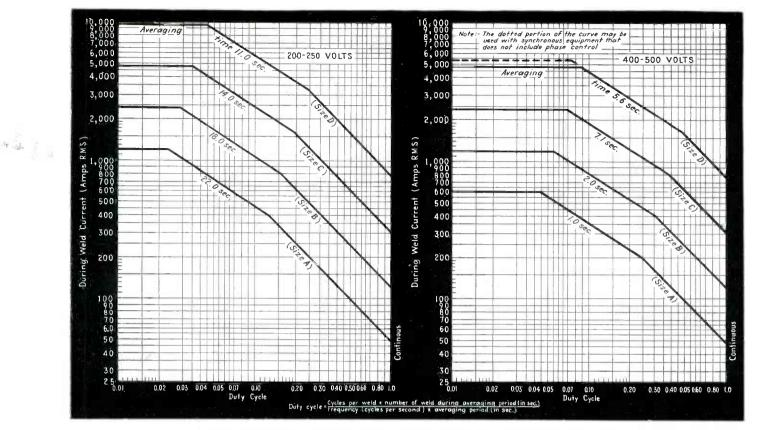
FIG. 2—Rating curves for four typical ignitron tubes used in welding control equipment. Data at the left is for 220 while that at the right is for 440-volt supplies
