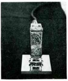
Fig. 2—Typical tracer unit. Note yoke supporting weight and establishing a reference level for the diamond point at the bottom, surface pressure adjustment knob at the top
