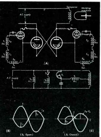
FIG. 5-(A) Phase control added to Fig. 1B. The amount of current that will flow to the welder depends upon the adjustment of  $R_1$ . (B) Voltage and phase relations with  $S_1$  open. (C) Voltage and phase relations with S<sub>1</sub> closed and the tubes passing current
