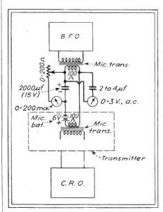
Simple "dummy microphone" setup for testing transmitter speech amplifier and modulator performance in production age should be sufficient to modulate the transmitter 100 percent, indicated by a cathode-ray oscilloscope connected to the transmitter output circuit in a conventional manner.
