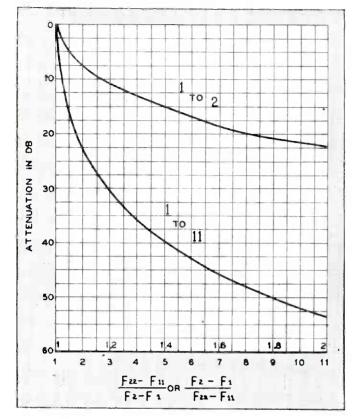
Fig. 2—Curve showing attenuation of band pass filter, without taking into account resistance in coils or condensers
