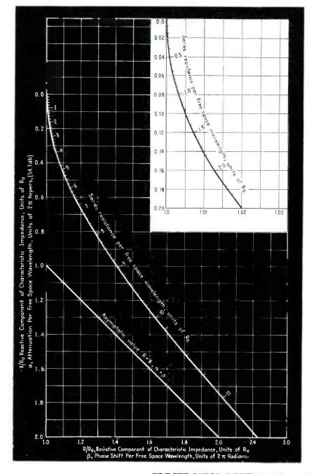
The attenuation is 0.0553x54.7 =3.03 db per wavelength. For the power to be reduced to 1/10 of its initial value or 10 db, the length of the line must be 10/3.03 = 3.3 wavelengths = 33 meters. This length of wire will dissipate 360 of the 400 watts fed into it. The other 40 watts must be taken up by a terminal resistor. A 1.5 inch spacing of the wires is needed to give the impedance characteristics indicated above.
