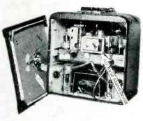
When the radio station goes off the air, the alarm automatically goes on, creating a loud, penetrating signal in the radio, warning one that an air-raid alarm is in order. The unit is supplied complete, in a compact case.
