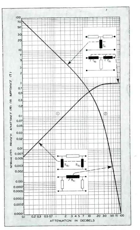
Fig. 5—Graph showing the normalized impedance or admittance for the series and shunt arms of T and  $\pi$  networks. Curve 1 applies to shunt elements of  $\pi$  network or series elements of T network, while curve 2 refers to shunt elements of T network or series elements of  $\pi$  network. The values obtained from this graph must be multiplied by the impedance level for which the symmetrical attenuator is designed
