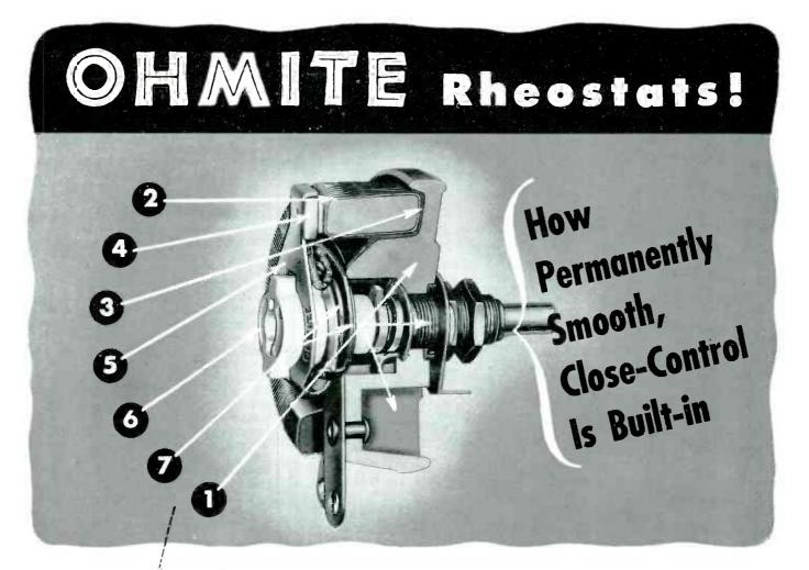
The cut-away view shows a number of the important features which make Ohmite Rheostats especially suitable for today's exacting requirements in industry, and in planes, tanks, ships. 1. Compact all ceramic and metal construction. Nothing to shrink, shift or deteriorate. 2. Wire is wound on a solid porcelain core. Each turn is a separate resistance step, locked in place and insulated by Ohmite vitreous enamel.
