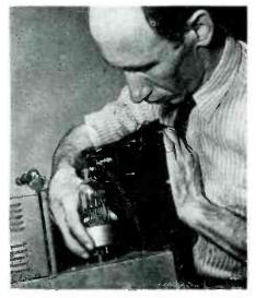
Fig. 2—The heart of the system, a special half-wave rectifier tube with gas intake and exhaust ports
