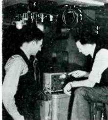
A G-E photoelectric color register control installed on a press in the plant of New York's Neo Gravure Printing Company is checked for synchronization by means of a cathode-ray oscilloscope
