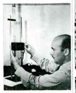
Dr. A. A. Bates of Westinghouse demonstrates P. R. Kalischer's device that quickly determines grain size of metallic powders having particles as small as 1/25,000 inch. Mixed with a liquid in a long glass tube, the particles intercept a light beam directed into a phototube as they settle. The rate at which the solution clears up, indicated by anode current change through a milliameter, gives comparative data
