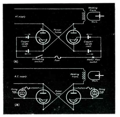
FIG. 1—(A) An electronic welding contactor without phase control or timing.
