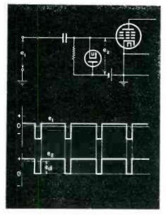
Fig. 18—Circuit for operating pulse waveforms from a fixed level
