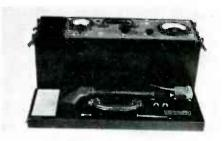
Fig. 3—The complete instrument, with cover removed. Tracer head, extra "yokes" and accessories may be seen in the foreground
