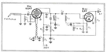
Fig. 2—Schematic wiring diagram of oscillator and discriminator of f-m phonograph pick-up recording system
