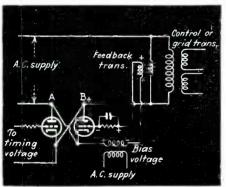
Fig. 6—A "trailing" tube control circuit
