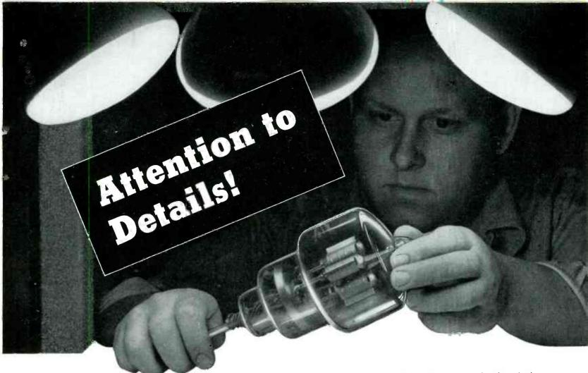
Near technical perfection is achieved through use of scientific instruments but the trained eyes of skilled workmen inspect completed units before they are passed along to the pumps
