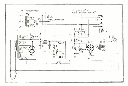
Circuit of automatic filament control device. Condenser  $C_{\rm i}$  should have low leakage and in the WQOC unit is oil filled
