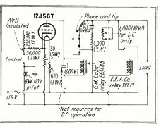
Schematic of electronic relay suitable for operation on a.c. or d.c.
