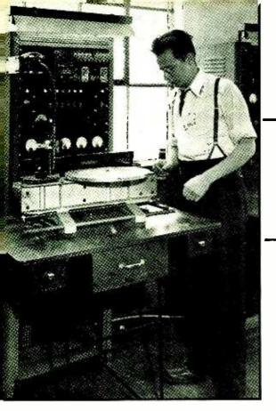
The Fluxgraph in use. The turntable carrying the coil under test may be seen at the left. A paper disc is in place on the turntable at the right
