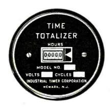
by a long-life synchronous heavy-duty self-lubricating motor, connected through gears to a five digit hour counter. The visible totalizer gives a record up to 10,000 hours.
