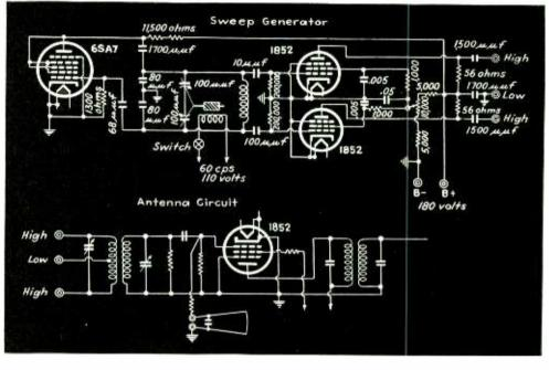
Fig 1. Circuit diagram of the sweep generator together with typical band pass amplifier tested by its means
