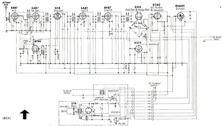
REPEATER—116-119 Mc amplitude modulated receiver. One or more of these are used at each of the six hilltop stations. Several interchanges and a majority of radio-equipped maintenance buildings use one apiece. (37.5 Mc amplitude modulated receivers employed at repeater stations, not diagrammed in these pages,
