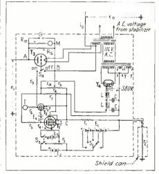
Fig. 2--Circuit of the electronic stabilizer
