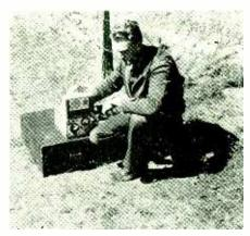
Portable 2726 kc 'phone transmitter-receiver used by Montana Power line patrolmen. It runs 2<sup>1</sup>/<sub>4</sub> watts output, weighs 22 lbs with batteries and antenna. The box on which the unit stands contains the batteries and antenna reel
