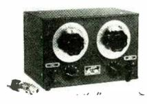
CFR testing engine or can be applied to studies with other engines for vibration and explosion phenomena. Model 2300 filter covers the range from 2000 to 8000 cps, and when used with Model 3000 pickup and cathode-ray oscillograph, it immediately indicates presence of detonation.
