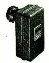
tions of ambient light and at various distances from a street lamp. The specially designed optical system on this unit makes it relatively insensitive to light from any source other than the street lamp which it is observing. A time delay is designed into the circuit of the control to make it independent of momentary fluctuation and flickering of the street lamp. It is operated from a 115 volt, 60 cps, a-c line. It is listed at \$81.50.
