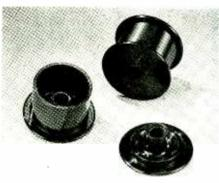
Plastic replaces aluminum in a new tungsten wire spool developed by Callite. Tungsten Corp., and at a saving of 20 percent. The spools are molded by Universal Plastics Corp. The Bakelite material is made in two sections which are fitted together and cemented to insure a permanent bond
