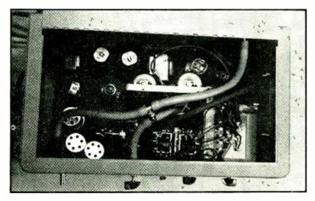
Inside view of the unit housing the amplifier, power supply, thyratron and relays
