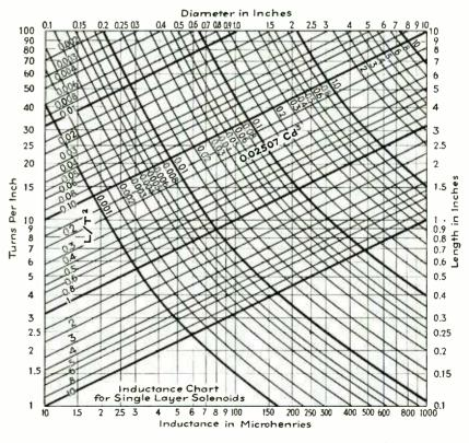
Graphical plot connecting all inductance factors for single layer coils and sufficiently accurate for most purposes
