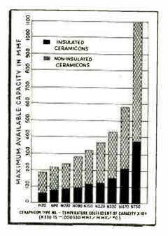
THE inherently stable retrace characteristics of Erie Ceramicons with respect to temperature insures dependable compensation for frequency drift. When properly used, one of these small, silver-ceramic condensers will accurately compensate for drift caused by temperature changes in any number of components in the circuit.
