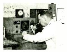
A 30 watt fixed station in operation in a natural gas pipeline dispatch office. Normally operated from the 110 volt a-c lines, all of these stations have emergency power supplies
