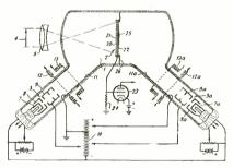
tralizing spurious signals generated by one of the electron beams. H. A. Iams, RCA. Dec. 21, 1940. No. 2,269,588.
