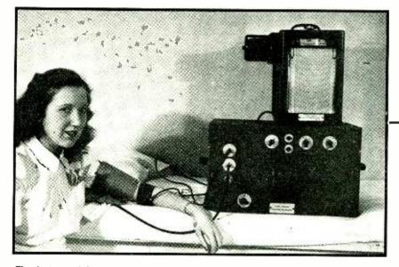
The instrument in use, cuff on patient's upper arm and stethophone strapped to forearm. Amplifier, power supply, control thyratron and relays are contained in the lower unit, while the modified dynamic speaker structure driving the sound actuated pen may be seen projecting to the left of the upper unit housing the pressure recorder
