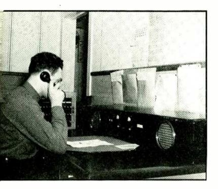
MIDWAY PATROL HEADQUARTERS—Many of the messages transmitted over the turnp:ke communication system originate at this "shuttle" relay point. One meter on the panel of the control unit illustrated indicates r-f when the local 116.95 Mc transmitter (in an adjacent room) is in use. The other is a modulation level indicator. Receivers at The Midway are tuned to 37.5 and 33.94 Mc
