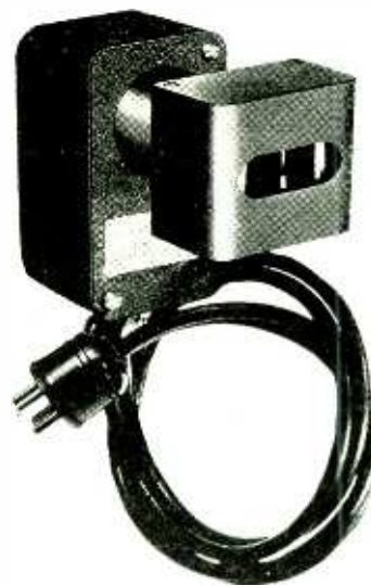
Fig. 1—Photoelectric scanner, combining light source, converging lens system and two phototubes in one housing
