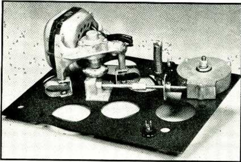
FIG. 5—Bottom of the chassis with the bottom side up. Note the motor mounting and the cutting-head arm drive shaft. Accurately spaced grooves are produced 200 to the inch
