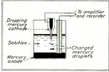
Diagram showing the principle of operation of the dropping mercury cathode
