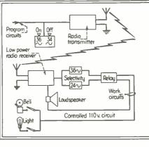
Fig. 1—Block diagram of the transmitter-controlled receiving system
