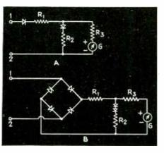
Fig. 1—Fundamental half-wave circuit (Å) and full wave bridge rectifier circuit (B) for straightening out the characteristic of the rectifier
