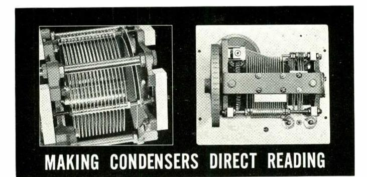
A VARIABLE AIR CONDENSER with semicircular rotor and stator plates can be made to have remarkable linearity over about 80 per cent of a half turn. When used with calibration curves or charts, the accuracy obtained is so high that for many years manufacturers were discouraged from attempting to make condensers direct reading.
