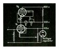
Fig. 2—The basic circuit of the voltage integrator using two pentodes and a voltage regulator tube
