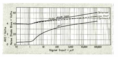
Ideal and realized characteristics of the noise silencer circuit
