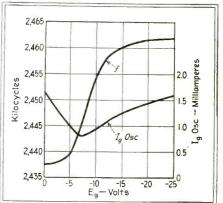
Fig. 2—Variation of oscillator frequency and oscillator grid current of the circuit shown in Fig. 1 as the modulating grid voltage is varied
