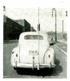
when used in conjunction with radio communication equipment on all types of military and commercial mobile vehicles and on boats. The manufacturer states that its advantages are that it permits a shorter or lower antenna to be used without loss of operating efficiency, and it provides greater efficiency when it is the same height or length as would be a conventional type antenna.
