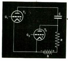
Fig. 1—Basic circuit of interval timer using two gas tubes and a condenser
