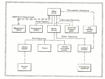
Fig. 1—Block diagram of the radio net used by the U. S. Forest Service in fighting a forest fire of the "conflagration" class—one whose area is 50,000 or 75,000 acres and whose perimeter is about 100 to 150 miles
