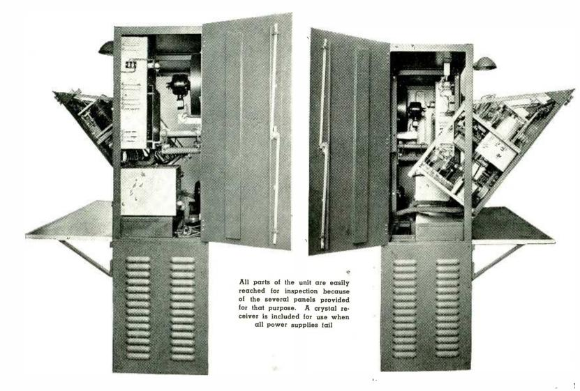
receiver, use of which is mandatory on all ocean going vessels, provides means for reception should all other devices fail. Though outmoded, and only dimly recalled by many in connection with the infancy of radio, the crystal receiver in its modern form with etched panel and double circuit tuning, is quite an effective and reliable device when used with a ship's main antenna.
