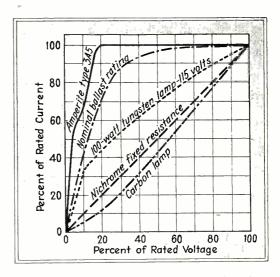
Fig. 2—Voltage-current characteristics of carbon and tungsten lamps compared with those of resistance regulators. Neither type of lamp offers much advantage over a straight dropping resistance whereas the regulator tubes provide regulation over a wide voltage range
