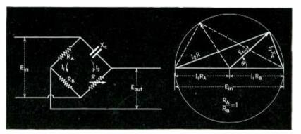
Fig. 1—The single reactance bridge phase shifter and its vector diagram. The output voltage is constant for varying phase angles when  $R_A = R_B$
