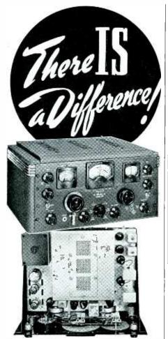
Try a Hallicrafters Super Skyrider, Model SX-28 and know the difference! — in operation, performance and stability. This 15 tube, 6 band communications receiver delivers dependable results, even under adverse operating conditions. Covers 550kc. to 42mc. The controls are arranged to give effortless tuning.
