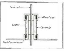
Fig. 4—A metal-ceramic-solder joint made without matallizing the ceramic
