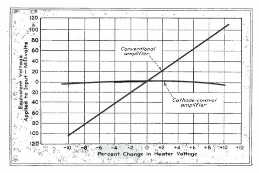
Fig. 5—Manner in which changes in heater voltage affect the equivalent input voltage applied to a conventional amplifier and to the cathode control amplifier described in this article
