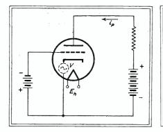
Fig. 6—Equivalent circuit of vacuum tube showing fictitious interval voltage, V, representing equivalent input voltage having the same effect as that produced by change in heater voltage
