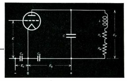
Fig. 1-Simplified circuit diagram of a triode radio frequency power amplifier
