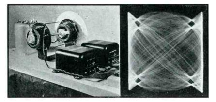
(Left) Fig. 11—Laboratory model of the 360-degree phase shifter whose circuit is shown in Fig. 8. (Right) Fig. 12— Lissajous figures taken with the 360-degree phase shifter
