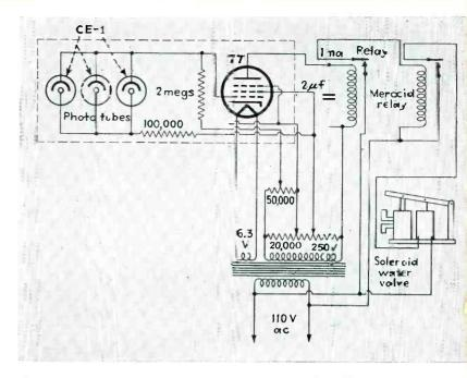
Circuit diagram of the infrared sensitive photoelectric relay. The three phototubes connected in parallel are mounted within a Pyrex glass cylinder. (Below) The ore moves from right to left on the pan conveyor. The water spray  $(\overline{A})$  is mounted away from the phototubes (B) to permit the ore to reach it before the water flows
