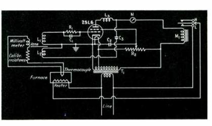
Schematic wiring diagram of the electronic pyrometer control unit
