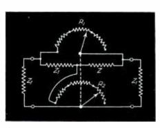
Simple voltage dividing network having given input impedance and specified loss, design data for which is worked out as Problem I
