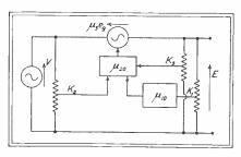
Fig. 10—Block diagram illustrating that the use of a feedback amplifier reduces variations in a regulated power supply
