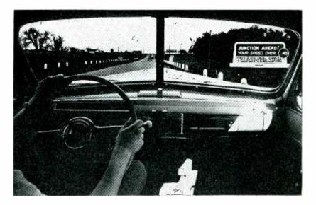
When a car approaches this automatic sign a photoelectric speed measurement circuit informs the driver of his speed
