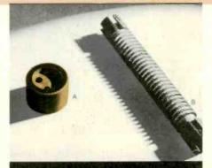
A — Connector plug — sawed, turned, and drilled. B — Coil form — turned, milled, and threaded.
