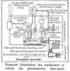
recorder is used For controlling the temperature of the anti-freeze solution, the tank is cooled with coils of a small domestic refrigerator and heated with suitable strip heaters. As the cooling system reduces the temperature of the solu-
