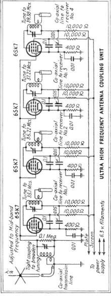
Circuit diagram of antenna coupling unit
