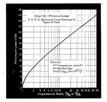
The minimum loss of any pad inserted in a circuit is given in decibels for impedance ratios,  $Z_1/Z_2$ , of from 1 to 100. The range may be extended for values of from  $Z_1/Z_2 = 0.01$  to  $Z_1/Z_2 = 1.0$  by forming the ratio  $Z_2/Z_1$  which will be greater than unity
