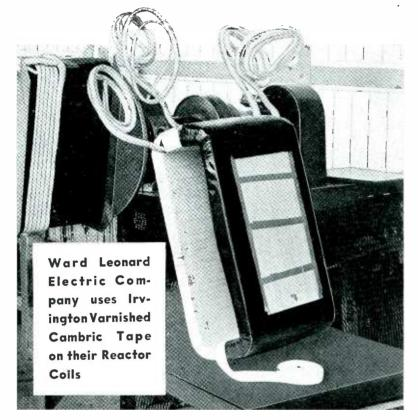
Here is an insulation that is pliable, tough and highly resistant to abrasion, moisture, acids, and lubricating oils. Surfaces are uniformly smooth. Dielectric strength is excellent. Furnished in dry, tacky and oily finishes.
