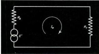
If  $R_b$ , the apparent resistance, is large so that  $X_L/R_b$  is small compared to  $1/Q_T$ ,  $Q_b$  will approach  $Q_T$ as a limit and the selectivity of the entire output circuit will approach that of the tank circuit alone. Usually  $X_L/R_b$  is comparatively large, making  $Q_b$  much less than  $Q_T$ .
