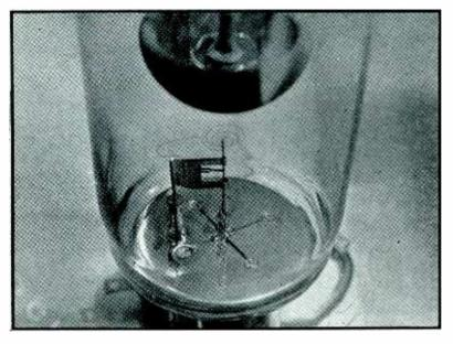
Fig. 4—View of pool cathode with floating starter assembly
