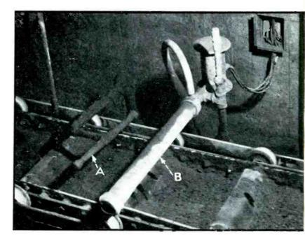
The wall-mounted relay unit. Note that the sensitive relay is enclosed in glass for protection against dust particles commonly found at an ore treating plant
