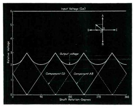
Fig. 9—Voltage curves of the 360-degree phase shifter showing variation in output voltage as the phase is shifted
