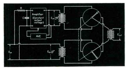
Fig. 10—Circuit of a 360-degree phase shifter which is independent of frequency
