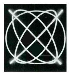
Fig. 13—Composite Lissajous figures showing constant input voltage and changing output voltage of the circuit of Fig. 10
