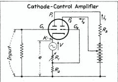
Fig. 7—Fundamental circuit of cathode control amplifier
