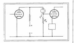
Fig. 12—By replacing the resistor, R<sub>1</sub> of Fig. 11 by a gaseous discharge tube, improved operation of the d-c amplifier is possible using a single voltage supply
