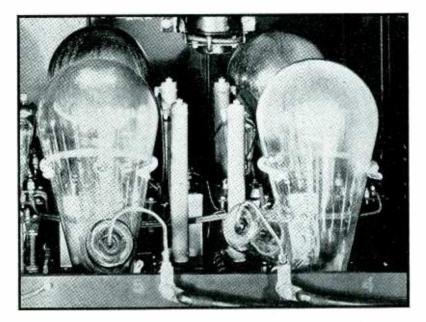
Fig. 5-Assembly of tubes with dielectric igniter, as used in industrial equipment
