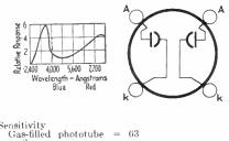
Sensitivity Gas-filled phototube = 63  $\mu_a/lumen$ Vacuum phototube = 10  $\mu_a/lumen$ Operating Voltage = 90 v
