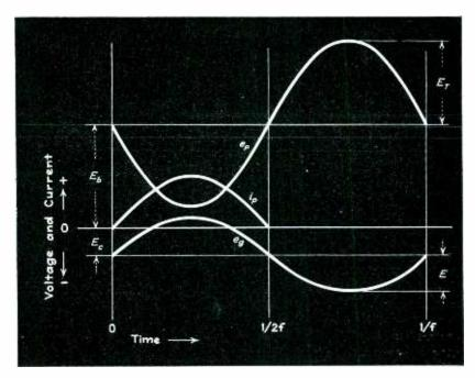
Fig. 2-Voltage and current relations in a triode power amplifier
