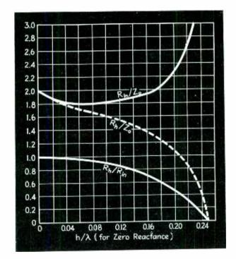
Fig. 5—Graphical data for designing a resistor to have zero reactance at a given frequency
