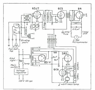
testing the lubricating qualities of oils. The loss of kinetic energy manifests itself through the decrement of rotational speed, so an apparatus was built which made it possible to accurately measure rotational speed from several hundred revolutions per minute to zero occurring during a time of several minutes.
