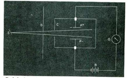
Fig. 5—Rough setup for measuring intensity of x-ray ionization. The x-rays flow through the opening in the lead sheet D into the chamber C where ions are formed. The ions migrate to the charged plates to cause a current flow which is measured by the galvanometer G
