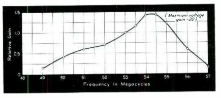
Fig. 4—Overall response characteristic of the television preamplifier, using damping resistors of ohms. Over the picture sideband, the gain varies about plus or minus 3 db, with a maximum gain of 20
