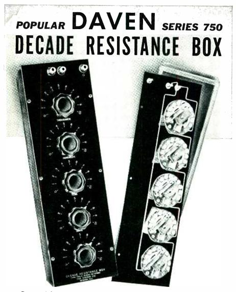
Designed for use as Laboratory Standards, as components in Bridge Circuits, and in other types of precision measuring equipment . . . the Decade Resistance Boxes are complete assemblies consisting of two or more Type 225 DAVEN Decade Units mounted on an engraved metal panel and enclosed in a shielded walnut cabinet.
