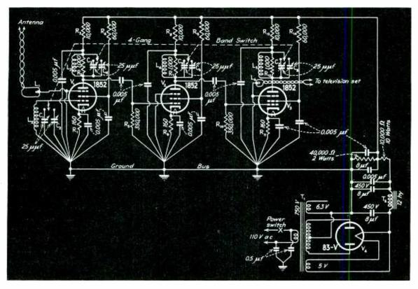
Fig. 2—The circuit diagram of the amplifier. By varying the values of the resistors shunting the tuned circuits, the gain may be varied approximately inversely as the bandwidth covered
