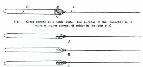
Fig. 2—Typical imperfect joints in the knives. The presence of less than the normal amount of solder causes the knife to be rejected
