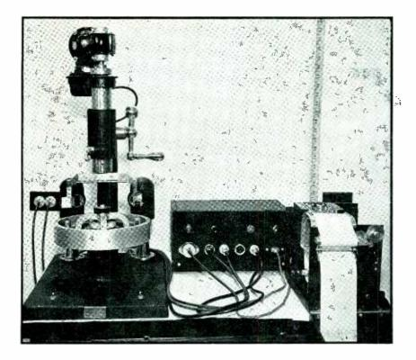
tube, a decagonal mirror mounted directly on the flywheel, an amplifier and the precision 60 cycles per second fork, and a Brush two-element crystal pen recorder. One face of the mirror is partially masked so as to identify every full revolution of the wheel and to make easier the counting of a long series of pulses. The completed apparatus is shown in Fig. 8.
