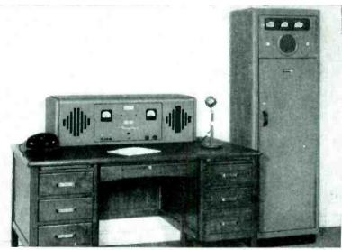
Motorola 250 or 500 Watt Central Station F-M Transmitter-Receiver and Remote Control Console
