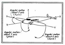
Fig. 1—An airplane has freedom of motion about three axes and is controllable by remote means in each of them
