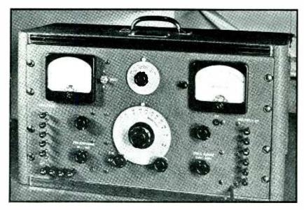
External appearance of the generator. Push button selection of the audio modulation frequency and output voltage level is provided
