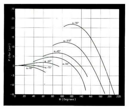
Fig. 6—The output voltage correction factor, P, versus the angle of conduction for cases where the rectifier resistance is appreciable
