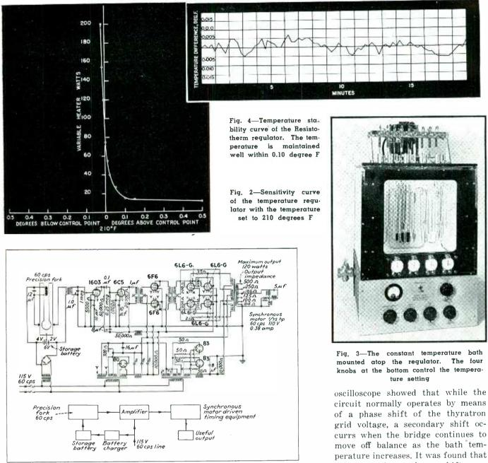
Fig. 5-Circuit diagram of the precision timing source for 60 cycles per second current. This unit is capable of driving 48 magnetic counters calibrated in seconds and tenths of seconds
