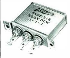
Aerovox also offers a line of midget rec-tangular-can oil-filled condensers, such as this Series 18 designed especially for use in aircraft and marine equipment. Corro-sion-proof can with special immersion-proof terminals. Choice of terminals at top or bettom of can.
