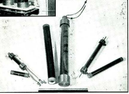
ductors when the resistors were immersed in water for cooling purposes. Resistors of the carbon rod type also have poor frequency characteristics, particularly in the higher values.
