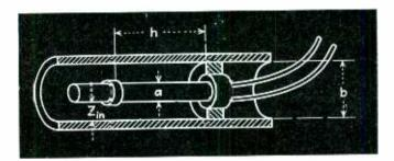
Fig. 4.—Structure of the "coaxial" water-cooling assembly. The water enters and leaves the assembly at ground potential
