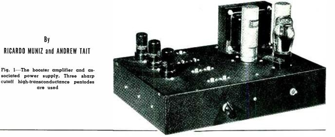
A description of a straightforward three stage r-f "booster" amplifier capable of an overall gain of from 20 to 1000 times, depending on the video signal bandwidth required. Useful in raising the sensitivity of television receivers in areas of low signal strength, or in overcoming transmission line losses
