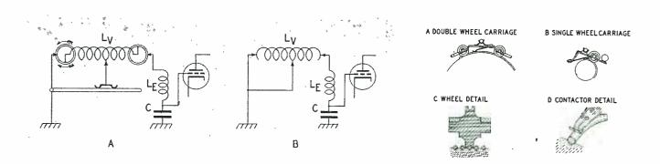
Fig. 1—Basic circuit of the Inductuner. Because the coil form rotates connections are made by continuous contact surfaces at each end of the coil form
