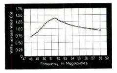
Fig. 3—Calibration curve of the communications receiver used to determine the overall gain of the television preamplifier
