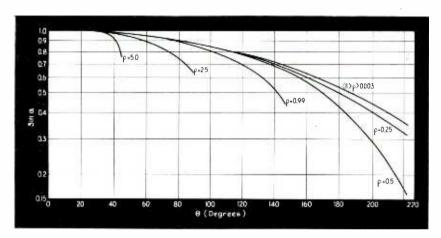
Fig. 5—The sine of the starting angle versus conduction angle
