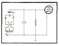
Fig. 1—Diagram of the basic circuit of the variable resistance crystal oscillator
