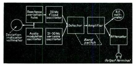
Fig. 1—Block diagram of the signal generator, showing the method of combining two oscillator outputs, one of which is frequency modulated
