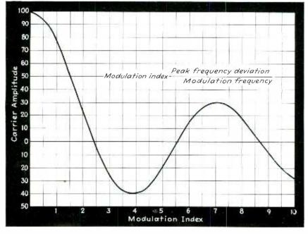
Fig. 2—Method of calibrating the frequency deviation scale of the instrument. The carrier voltage goes to zero periodically, as the modulation level and frequency deviation are increased (after Crosby)
