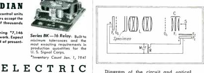
Diagram of the circuit and optical system of the photoelectric turbidimeter
