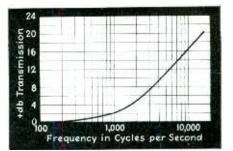
Fig. 3 — The standard pre-emphasis characteristic incorporated in the generator is removable by means of a selector switch, whenever overall "flat" measurements are to be made
