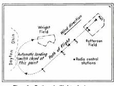
Fig. 3—Path of flight during an automatic landing
