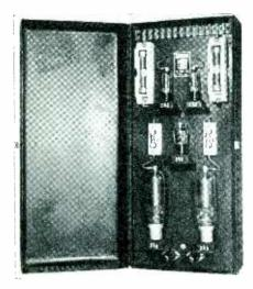
sizes. The synchronizer is housed in a dustproof steel cabinet approximately 30 inches high by 12 inches wide by 12 inches deep for wall mounting and is easily wired to any existing non-synchronous timer. An adjustment for any value of power factor in the welding transformer is provided.
