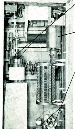
THE 892-R POWER amplifier tube, aircooled, is easily reached when the rear door of the radio frequency power amplifier cubicle is opened.
