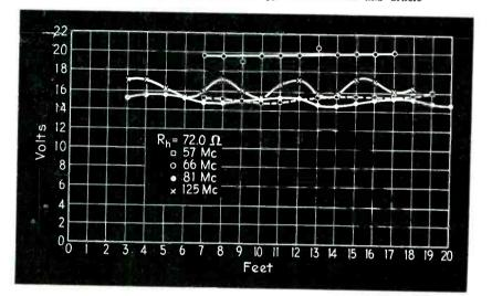
Fig. 8 — Characteristic impedance of a highresistance line, which simulates the watercooled resistor
