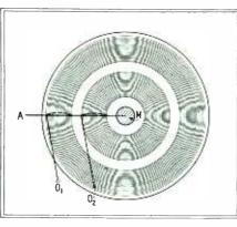
Fig. 1—Stereophonic record showing two sound-tracks
