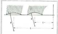
Fig. 2—The pickup arm of the inside sound track is shorter than the other
