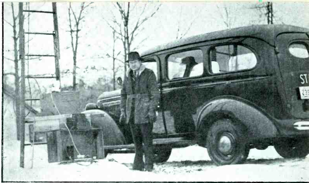
Fig. 2—Right, the original exploration transmitter, used for testing proposed sites in each troop area
