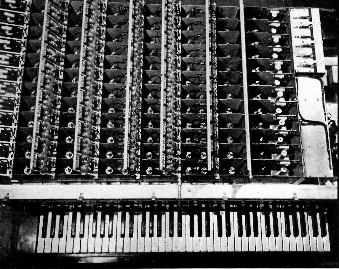
Fig. 1—Left, by the use of vacuum tube oscillators, the Novachord produces a wide variety of musical tones
