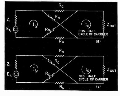
Fig. 12—Equivalent circuits for the ring modulator
