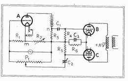
Fig. 2—Improved circuit, used to measure  $\mu$  of tube A
