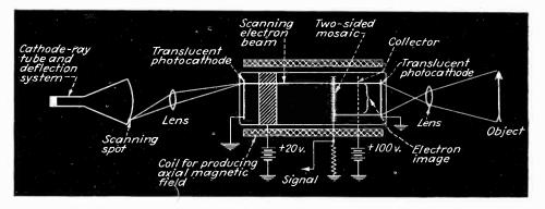
Fig. 6—Another developmental form of the tube used a two-sided mosaic, with image on one side and scanning electrons in the other. The flying spot of light was retained
