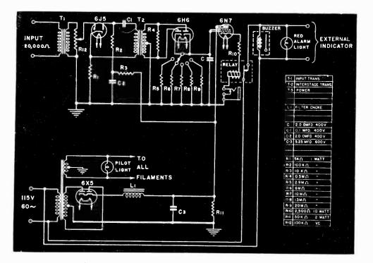
Circuit diagram of program failure alarm. Variation in the time delay before the alarm operates is provided by the adjustable diode load resistor and condenser
