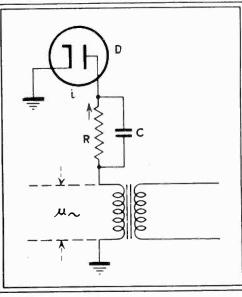
Fig. 1—Schematic wiring diagram of impulse detector
