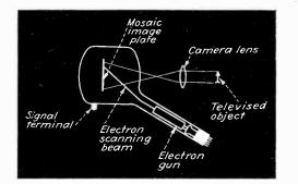
Fig. 1—Arrangement of the conventional iconoscope, now widely used as a pick-up camera tube
