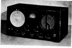
new receiver, model S-19-R, has six tubes including the 6K8G. Continuous coverage from 545 kc to 44 Mc is pro-
