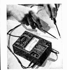
Independent of Battery Voltage Ranges-from .1 ohm up to 200,000 ohms
