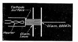
Fig. 7—In the present form of the Orthicon, this very simple electron gun is used
