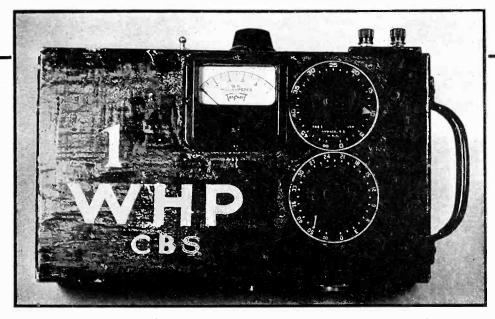
In the interests of portability, only two high-impedance microphone channels are used and the usual transformers which occupy much of the space are eliminated
