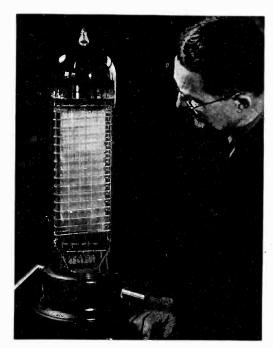
A three electrode vacuum tube of giant dimensions is specially constructed with filaments on the outside and plate on the inside. The plate is coated with fluorescent materials so that the operation of the tube can be determined visually
