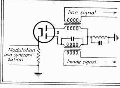
Fig 2—Double diode impulse detector circuit
