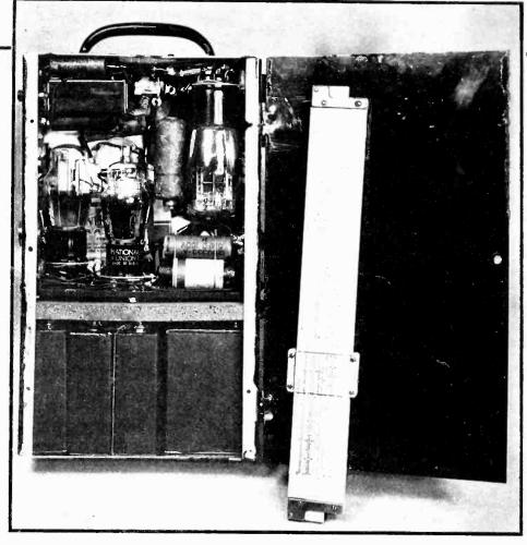
View of amplifier with cover open. Filament power is supplied by single 3-volt battery with a dropping resistor and the plate voltage is supplied by three small batteries. Four tubes of the 1.5 volt series are used
