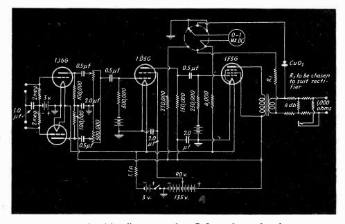
By the use of a 0-1 milliameter with a CuO rectifier and a three-way switch (top, above), it is possible to check the output level, the A voltage or the B voltage at any time
