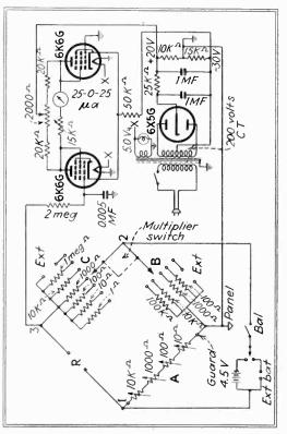
Fig. 2—Complete circuit diagram of bridge
