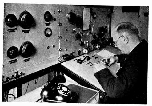
The apparatus shown here monitors the short and long waves and is used to indicate the source of short wave interference at the International Union of Radio Fusion
