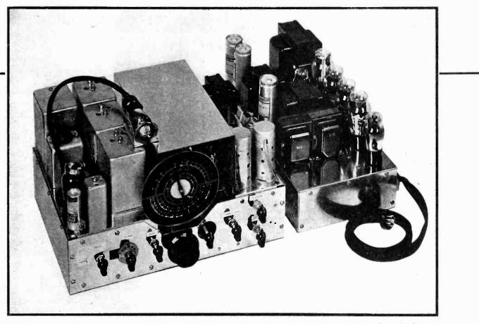
The receiver is contained in two chasses; the r-f and i-f units and first audio stage are in the left chassis and the audio power amplifier and power supply are in the right chassis. All controls and a heater transformer for the tuner tubes are mounted on the tuner chassis
