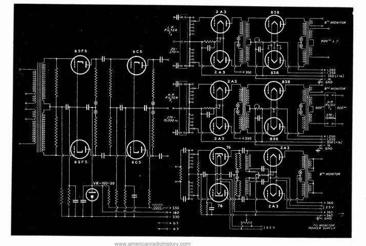
Circuit diagram of amplitier system. Each of four sound projectors is fed by a separate group of amplifiers
