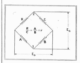
Fig. 1—Basic bridge circuit
