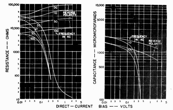
Fig. 2—Small-signal resistance and capacitance vs bias voltage of "Varistor" unit
