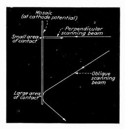
Fig. 3—When low-velocity electrons are used for scanning, defocussing occurs unless the scanning beam hits the mosaic perpendicularly
