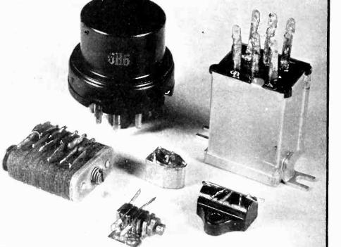
Fig. 3 --- Typical CuO rectifier structures, sizes shown relative to 6H6 double diode
