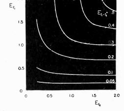
Fig. 11—Voltage levels for two carriers and difference frequency
