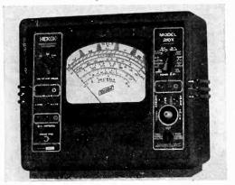
has ranges for measuring up to 10,000 volts. It will also measure currents up to 25 amperes, resistances up to 50 megohms, capacitances to 200 microfarads. A decibel range is included.
