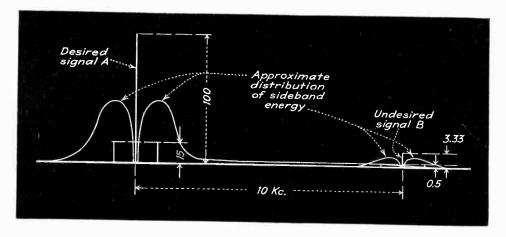
Representation of the relative strengths of the desired and undesired signals and their sidebands. The energy of the sidebands is concentrated in the region between 100 and 2000 cps
