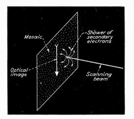
Fig. 2—When the high-velocity scanning beam hits the mosaic it generates a shower of secondary electrons which fall back on the mosaic, producing a spurious signal
