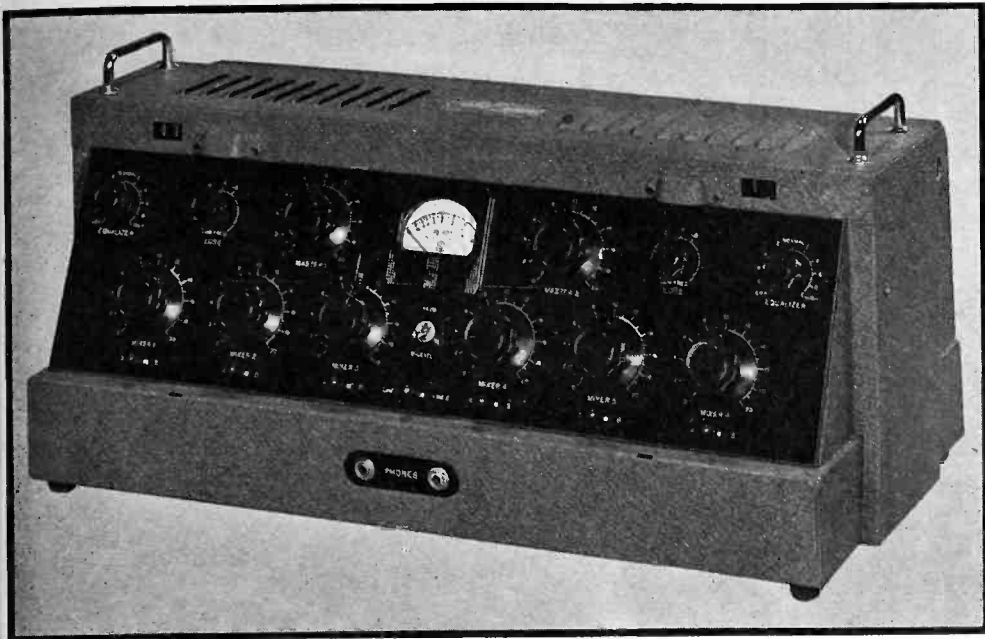
This mixer and preamplifier provides individual control over two lines. It is manufactured for broadcast station use by the Operadio Company
