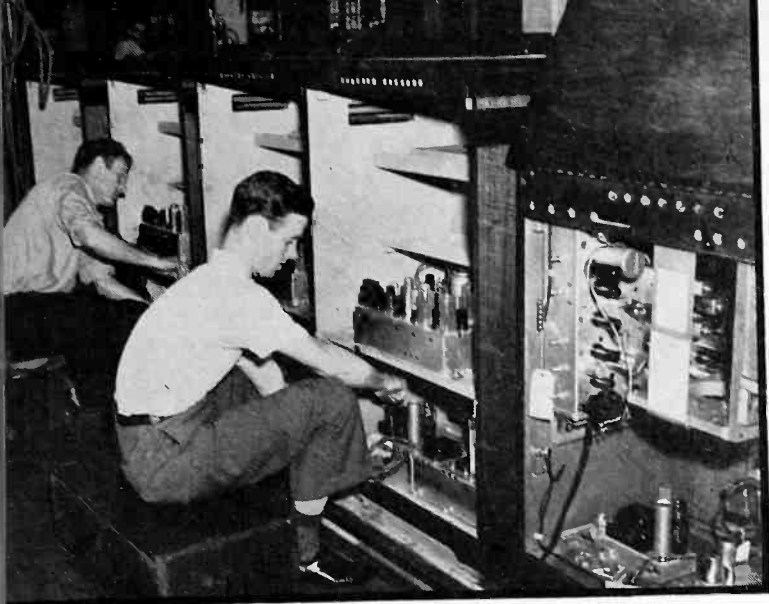
Installing the lower chassis (power supply) in a group of direct viewing consoles. The receiver at the extreme right is of the mirror-viewing type, with chassis mounted vertically
