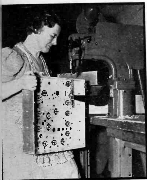
Sockets are numerous in a television chassis. Here the mechanical work of assembling the parts is completed before wiring
