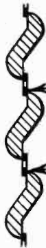
Louvres should be designed so that the flash shows as little as possible
