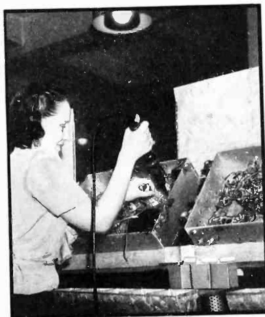
Wiring the chassis proper, one of the most complicated jobs in the radio field, is handled by the most experienced and capable operators
