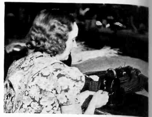
Wire stripper which burns off silk and cotton insulation from wire ends, in use at Stromberg-Carlson plant
