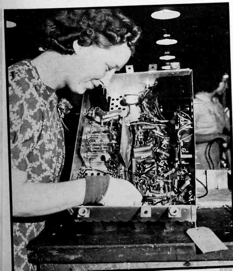
A final check-up of a nearly completed chassis is made by an operator who wears gloves to protect the parts from dirt and moisture. The wave-change switch and associated circuits are at the left
