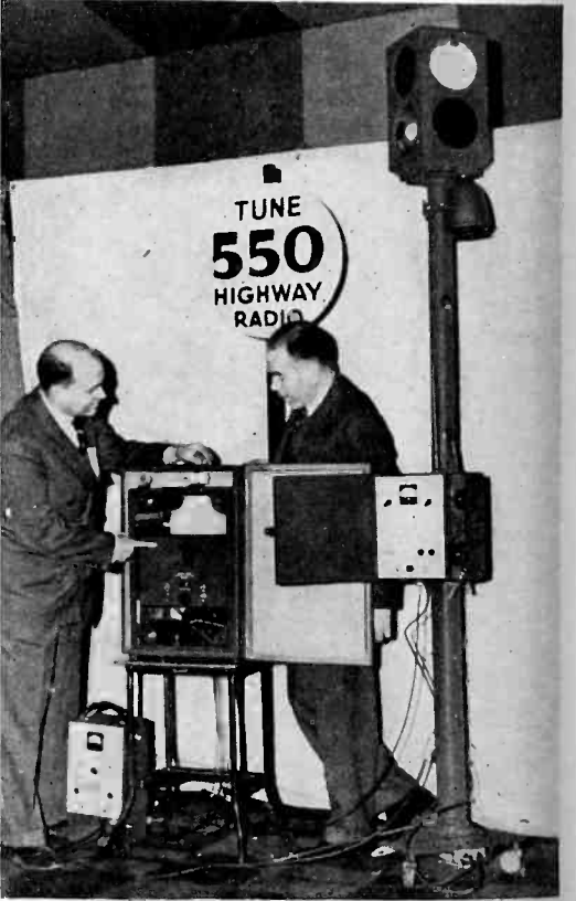
William J. Cox, left, and Dr. Miller McClintock, Director of the Bureau for Street Traffic Research of Yale University, are shown inspecting the robot radio policeman recently demonstrated before the Greater New York Safety Council. More effective control of traffic through the application of electrically operated equipment is expected to result from the installation of equipment such as this
