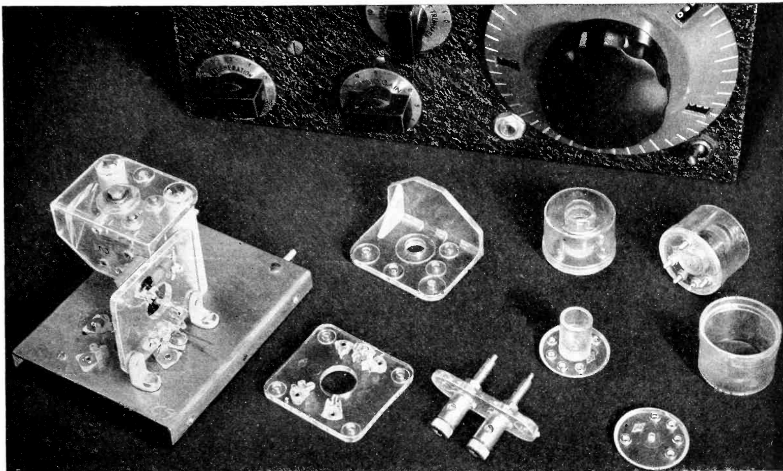
Tube sockets, condenser brackets, antenna terminal strips, and cases, forms and bases for coils in the new "110" National Co. Receivers are made from Bakelite Polystyrene. Molded by Thomas Mason, Inc.
