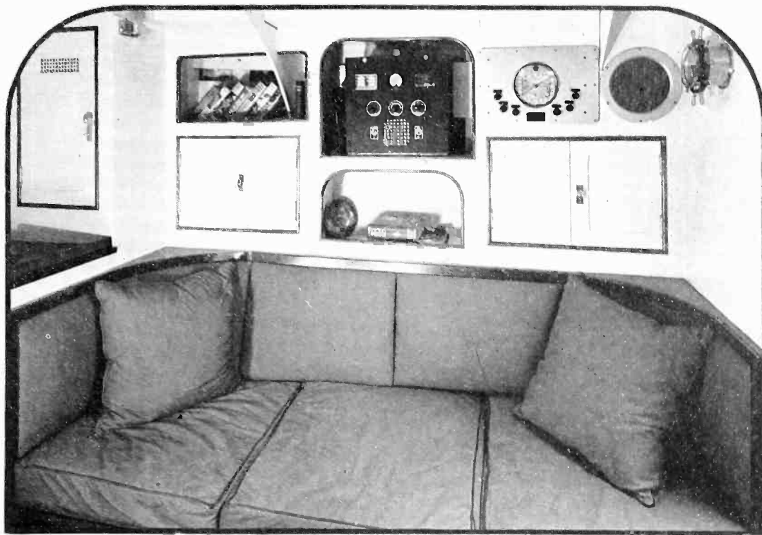
Salon of the Wakiva with 15 watt two way marine radio telephone occupying a convenient niche
