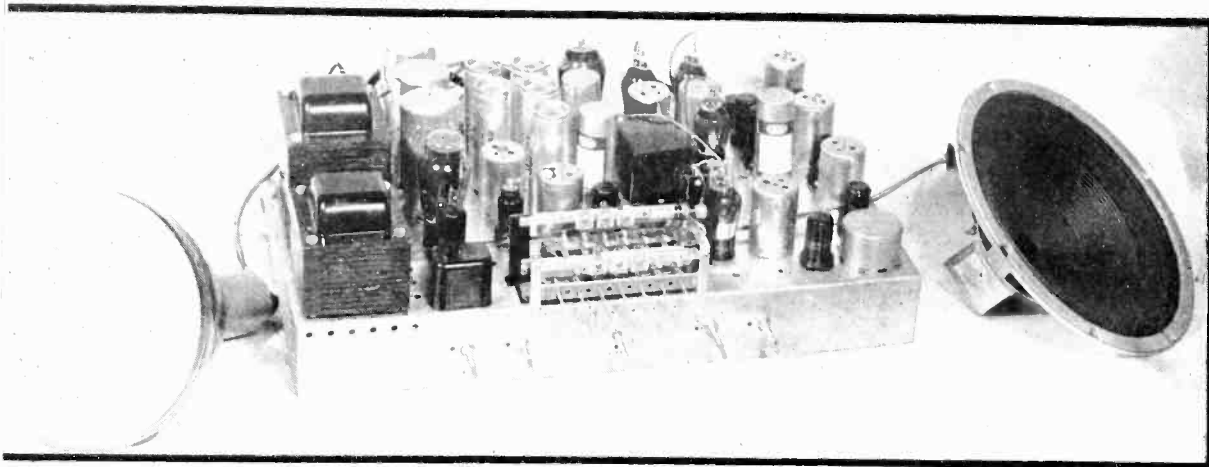
Fig. 3—Chassis of the 9-inch set manufactured by the General Electric Company, which employs a "short" tube of the magnetically-focused variety
