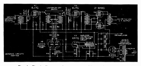
Fig. 1—Circuit diagram of program amplifier with automatic gain control
