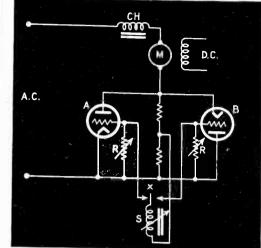
Fig. 2—Motor reversal and speed control of d-c motors are possible with this circuit
