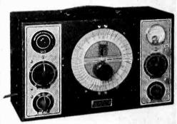
Verni Vider dial. With its accurately calibrated output of 1/2 to 100,000 microvolts at frequencies from 100 kc to 30 Mc, it provides an accurate yardstick of receiver over-all performance.
