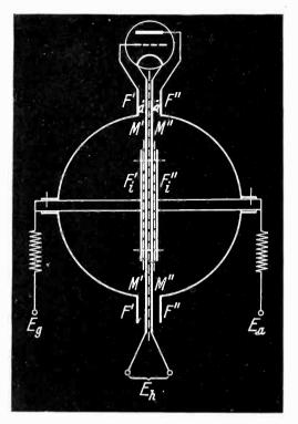
Fig. 6—Schematic circuit of oscillator with external tube
