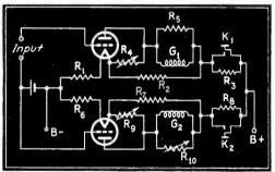
Fig. 1—Schematic wiring diagram of push-pull voltmeter
