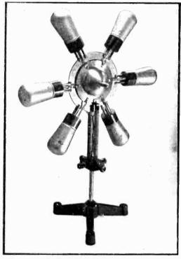
Fig. 7—Spherical tank transmitter with 6 external tubes
