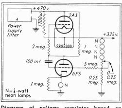
Diagram of voltage regulator based on Bousquet's design
