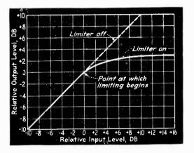
Fig. 2—Input-output characteristics of limiter circuit
