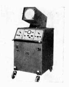
special cathode-ray oscillograph, Model 136-B, makes it possible to examine the wave form of minute impulses and to produce a large image on the tube for photographic purposes.
