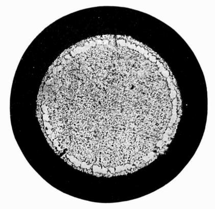
Fig. 2-Cross sectional diagram of carburized thoriated fungsten filament which has been partly decarburized. Magnification, approximately 300 imes
