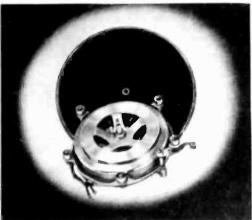
The motor is self-starting with stepless, smooth variation of speed over a wide range. One-shot lubrication through the shaft makes it unnecessary to remove the turntable when oiling. The motor is five-position rubber mounted, available in either 33 1/3 or 78 rpm, and is 4 in. high x 9½ in. in diameter furnished with a 12 in. Florentine bronze turntable.
