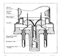
Base construction of the new RCA single-ended Twin Triode Amplifier isshown in this crosssection diagram. It also shows shield cone and cylinders for reducing inter-electrode capacitance,
