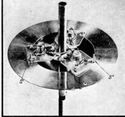
Fig. 5—Transmitter with three internal Acorn tubes. Above, (a) the internal arrangement. Right, (b) the external view
