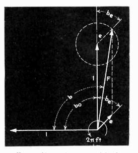
Vector addition of main signal (one) and echo (e) to show effects of amplitude and phase distortion (Wheeler)
