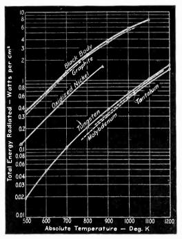
Fig. 3-Characteristics of suitable anode materials for electron power tubes
