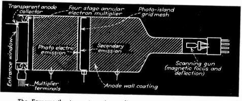
The Farnsworth storage-type image-dissector tube, which displays no shading signal and has ten times the sensitivity of the ordinary iconoscope
