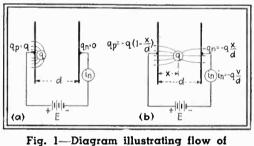
Fig. 1—Diagram illustrating flow of current in tubes operated at high frequencies
