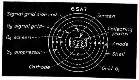
The electrode structure of the new single-ended pentagrid converter employs some of the principles of the beam power tube in obtaining better performance with one less terminal
