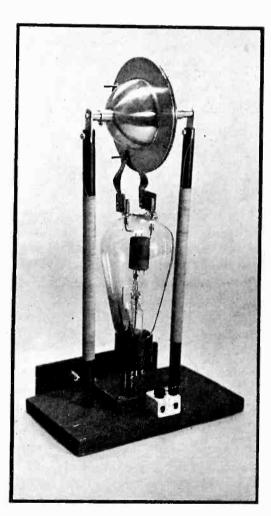
Fig. 3a—Single tube transmitter with RCA 834
