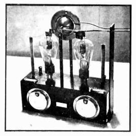
Fig. 8—Push-pull oscillator using RCA 834 tubes
