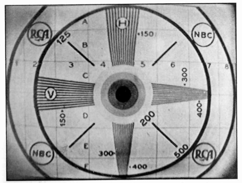
Fig. 2 Image of test pattern, actual size, as received from Empire State transmitter using complete receiver shown in Fig. 1
