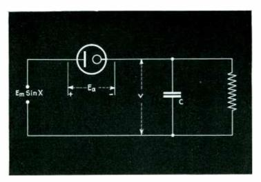
Fig. 6—Gas tube rectifier circuit having resistive and capacitive plate loading
