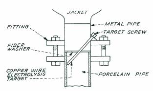
Fig. 5-Drawing showing how targets work
