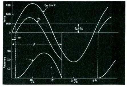
Fig. 4, left-Schematic diagram of half-wave rectifier having induc-tive and resistive plate loading
