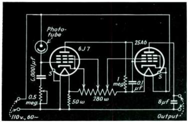
Fig. 3—A simple two stage a-c operated phototube circuit and amplifier functioning in a negative direction on the received light
