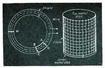
Fig. 4A (left)—Electrostatic shield in which loop winding is enclosed in metallic tube. Fig. 4 (right)—Electrostatic shield of woven gauze as used in broadcast receiver.
