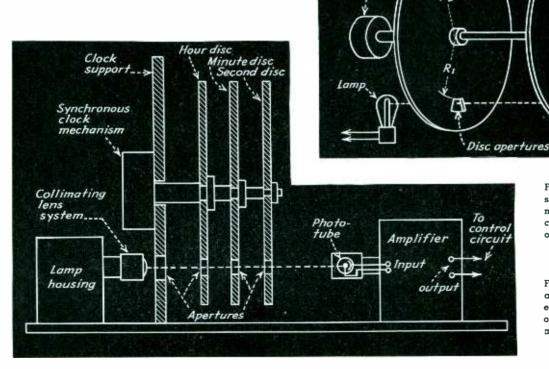
Fig. 1, left — Diagram showing the fundamental mode of operation of clock driven, phototube operated electric timing device
