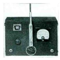
from a single dry cell mounted in the case. A wavechange switch for six bands and a phone jack for monitoring are provided. A damped meter indicates the relative radio frequency field strength.
