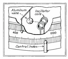
Arrangement of pick-up coils and aluminum vane
