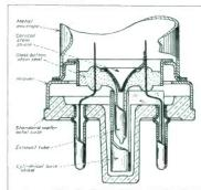
Base construction of the new RCA single-ended pentodes is shown in this cross-section diagram. It also shows shield cone and cylinders for reducing inter-electrode capacitance.
