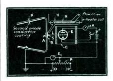
Fig. 1—Circuit showing method of measuring screen potentials of cathode ray tubes
