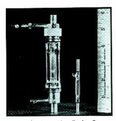
Announced coincidentally by General Electric and Westinghouse, a new 1,000-watt high pressure mercury lamp, shown at right above, is cooled by running water through a jacket surrounding the lamp. The water filters out much of the infrared but allows the ultraviolet and visible radiation to escape. The brilliance attained is about one-fifth that of the sun's surface
