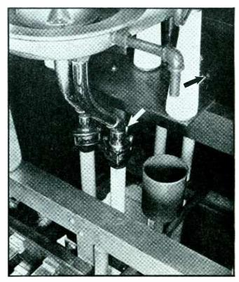
Fig. 2—Method of attaching the pipe to the water jackets.
