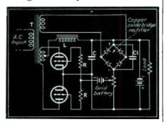
Fig. 2—Full-wave self regulated rectifier circuit
