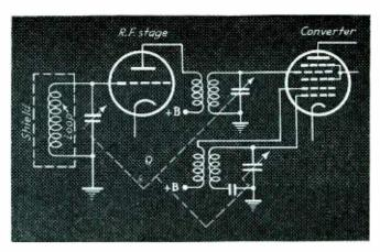
Fig. 5—Schematic wiring diagram of the input circuit for receiver having shielded loop for reducing electrical noise. Condenser tuning the loop is ganged with other tuning condensers.
