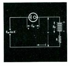
tive. The time angle of firing  $\alpha$  is  $\sin^{-1} k$ . The angle of "cut off",  $\beta$ , is  $(\pi - \sin^{-1} k)$ . Figure 3 illustrates the nature of the current function. It may be seen that the current flows in impulses which are portions of sine waves. The average, or d-c value of the anode current is
