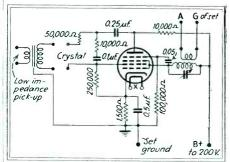
Fig. 1—Basic circuit of phonograph oscillator
