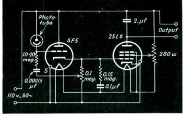
Fig. 4—Another simple a-c operated phototube control circuit operating in a positive direction on the light received by the phototube
