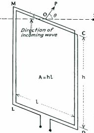
Fig. 1 (above)—Loop diagram for which equation (1) is derived.
