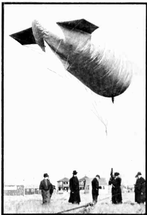
Supporting a quarter-wave vertical wire, this balloon indicated a new and better location for WBZ
