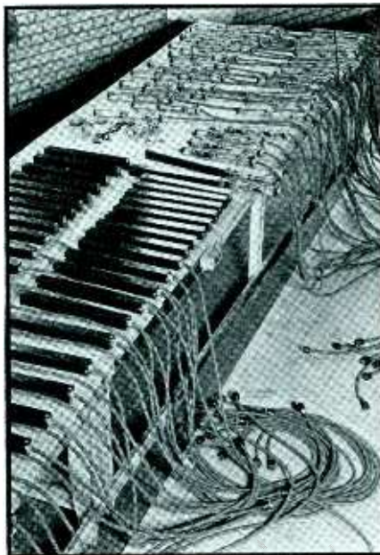
Each of these rod-like structures is a complete phototube relay, containing the phototube, amplifier tube and auxiliary components, designed by the Electronic Control Corp. of Detroit
