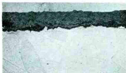
Micrograph of carbonized Nickel. The coating adheres tightly to the metal, and is not damaged by forming operations or by expansion of the metal at high temperatures.
