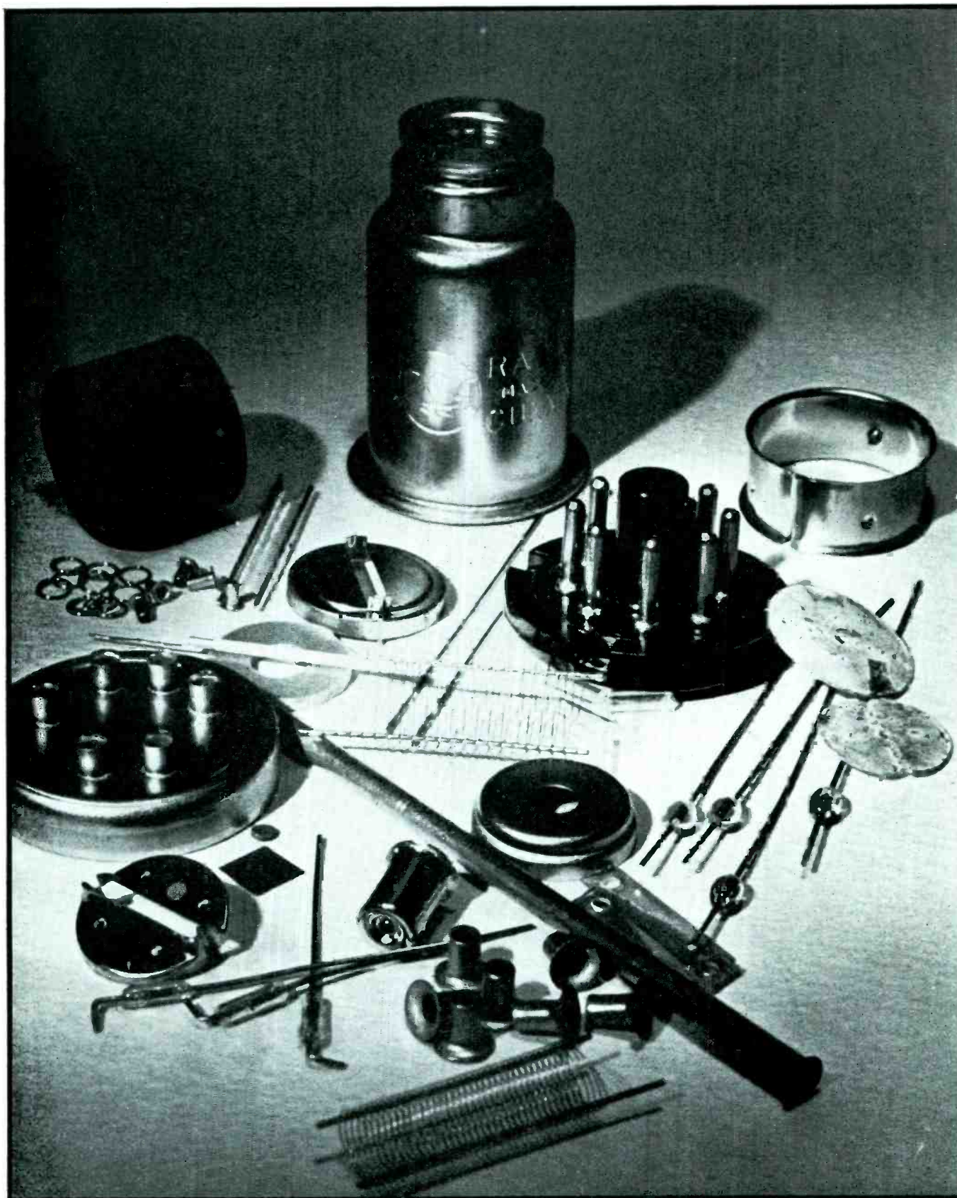
The works of a metal tube. A Leica photo by Arthur Van Dyck showing the 50-odd parts that go into the making of a metal-shell amplifier. Recent changes in design have changed somewhat the appearance of the header and certain of the smaller parts
