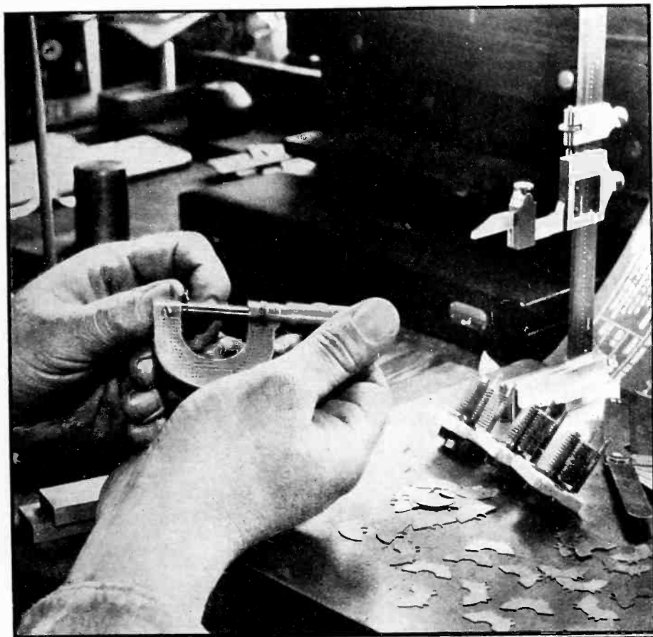
Checking accuracy of condenser plates with micrometer. In background is a vernier height gage and below is a thickness gage to measure air gaps
