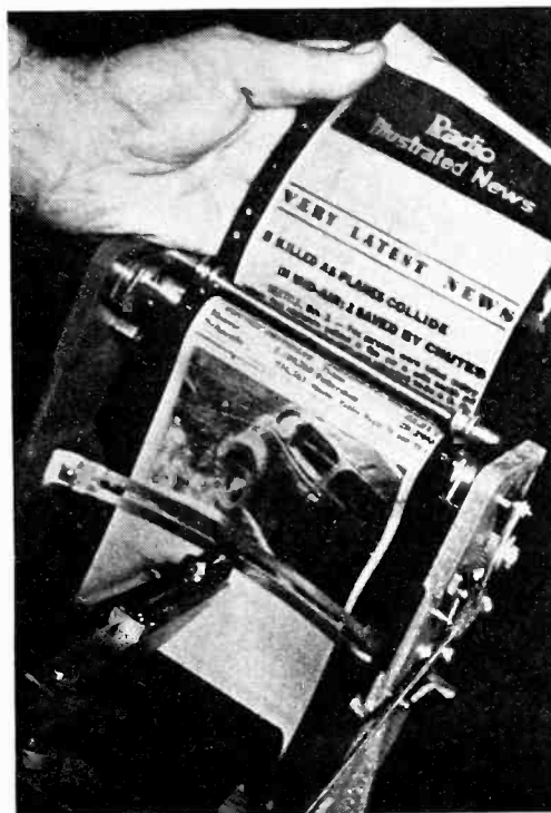
Typical printed matter as reproduced on home facsimile recorder. In order to show details of the recording stylus, the cover has been removed
