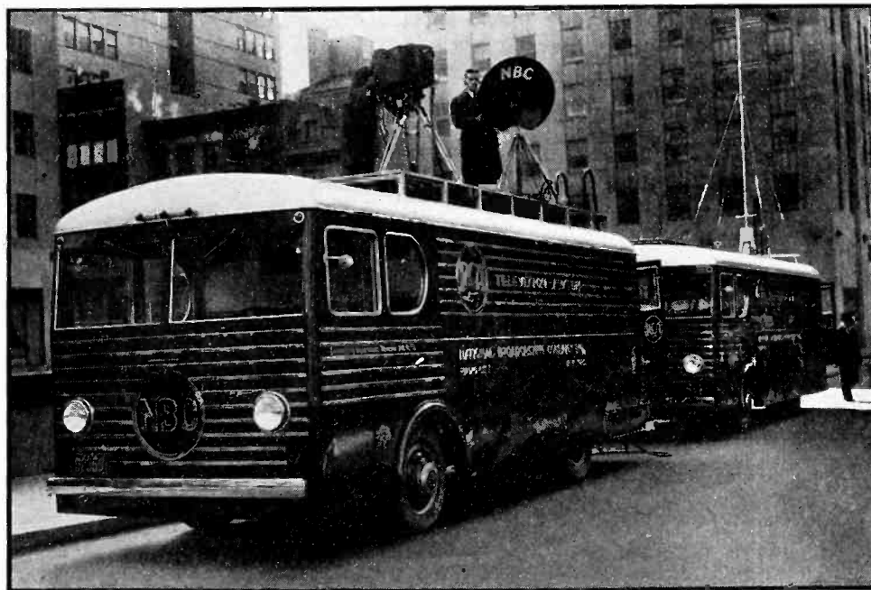
NBC's new portable television station, mounted in two "telemobiles", for relaying outside pick-ups to the Empire State transmitter. Platforms on the roof hold Iconoscope camera and parabolic microphone pick-up, while the antenna (on pole, rear truck) delivers the 177 Mc. signal to the main transmitter, either directly or through intermediate relays
