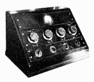
Control panel with four input microphone positions. The top panel contains the volume indicator, the middle
