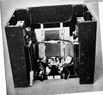
unique Screws hold more securely than machine screws in either inserts or tapped holes." It is no wonder that this manufacturer says—"Now when an assembly is to be made on any of our products we first consider Hardened Self-tapping Screws."
