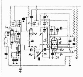
these circuits being coupled or connected with separate grid electrodes of a tube arranged in parallel electron streams, whereby varying bias on the grid controls their d-c potential. No. 460,055. E. K. Cole.
