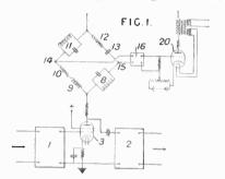
when the received frequency band is coincident with the predetermined pass band of the appropriate amplifier while any departure from tune causes the bridge to be unbalanced. Marconi Co. No. 462,328.
