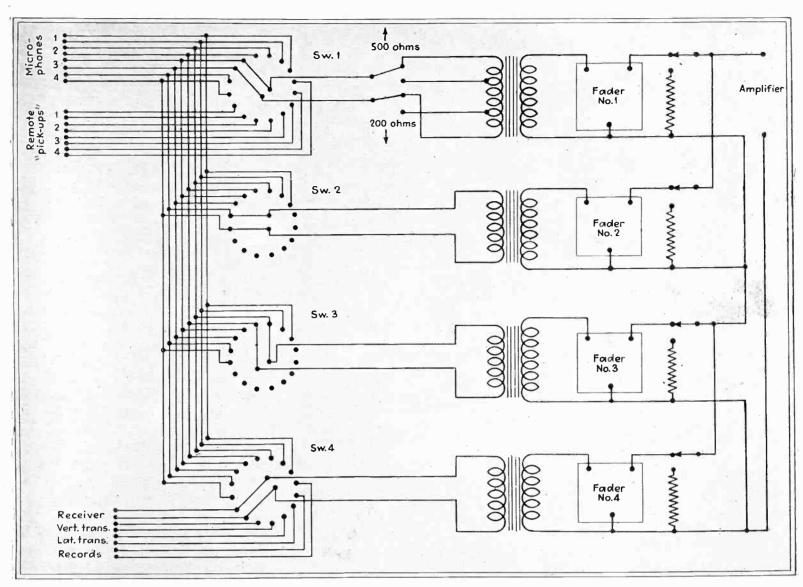
Schematic wiring diagram of the microphone control panel at KONO. The four switches at the extreme left replace patch cords and serve as microphone selectors. The resistors at the right are thrown into the circuit when the faders are not used to keep the input impedance to the amplifier circuit constant
