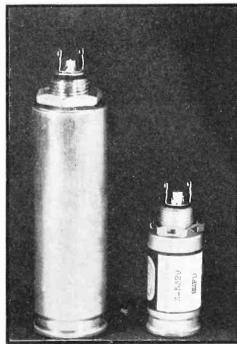
All manufacturers are reducing electrolytic sizes. These Solar units have identical capacity and voltage characteristics
