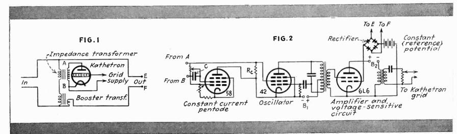
Fig. 1—Fundamental schematic wiring diagram for kathetron
