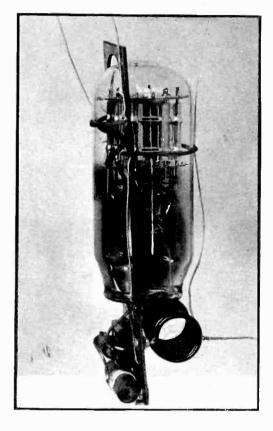
Transmitter used at Blue Hill. The tube, specially made for the purpose, contains two triodes (similar to type 30's but with 1.5 volt filament). It is powered by the batteries at lower left
