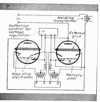
Fig. 3—Welding application of pool type mercury arc kathetron
