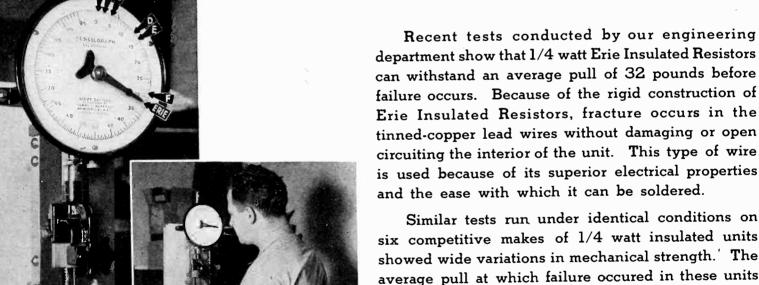
is indicated by the arrows on the testing machine illustrated at the left. Patented construction of Erie Insulated Resistors gives you this extra margin of safety against open-
