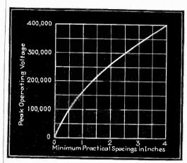
Electrode spacing for high voltage rectifiers
