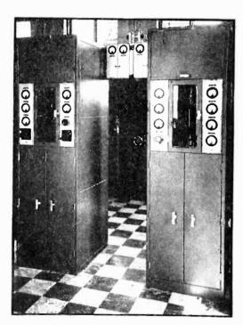
A feature of this low power (400 watt) Western Electric transmitter used in ship to shore communication is the ease with which frequency can be changed. By twirling the telephone dial, lower left meter panel of the right hand unit, any of ten carrier frequencies is automatically chosen
