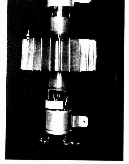
A 25 ampere kathetron tube with external grid
