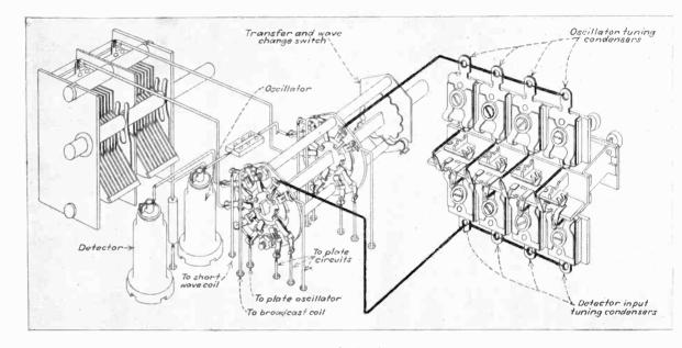
Fig. 5-Push-button condenser substitution system
