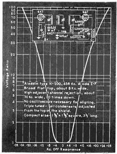
Characteristics of i-f transformer of interesting characteristics together with circuit and suggested
