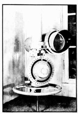
The indicator of this Telefunken direction-finding loop is a cathode ray tube, which gives an "average" reading in the presence of rapidly changing wave-front phases which occur during sunset and sunrise hours and which make for inaccurate aural indications
