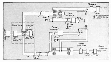
Fig. 2—Hybrid coil circuit through which two separate one-way radio circuits are combined into a single two-way communication circuit
