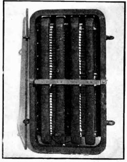
The inverse of the ribbon-type microphone, this German loudspeaker consists of four magnet coils which supply the field and two aluminum ribbons. The speaker is three feet high and operates with an input power of 1000 watts
