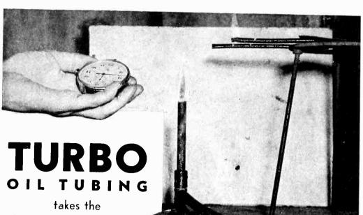
Photograph of test wherein TURBO Oil Tubing proved it burns 8 times slower than any other like product.
