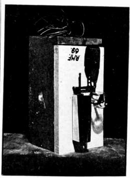
Complete radio meterograph without radiation shield
