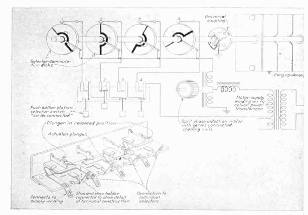
Fig. 3—Schematic of "homing" system employing series connection switch. Inset shows mechanical details of series-connected switch
