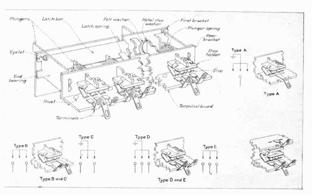
Fig. 4—Push-button selector switch, showing mechanical details and connection diagrams of five single row and one double row type
