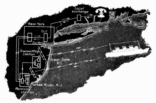
Fig. 1—Schematic diagram of the ship-to-shore communication circuit. The shore receiving station is at Forked River, the transmitter at Ocean Gate, N. J.
