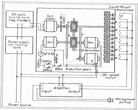
Block diagram of stroboscopic method of determining frequency
