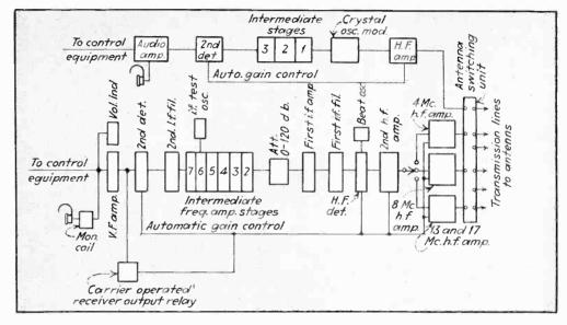
Fig. 3-Block diagram of the service receiver at Forked River
