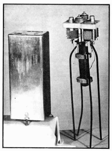
Double tuned air dielectric capacitor. Note the heavy ceramic insulation. A Sickles coil
