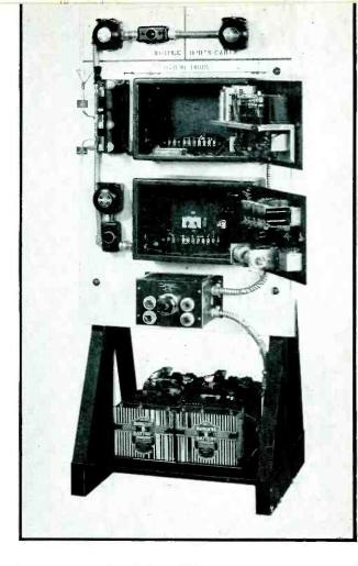
Two views of the Federal Telegraph (Mackay Radio) Auto Alarm, which times the distress signals mechanically. The upper unit is the receiver, the output of which controls the timer and counter in the lower unit. The alarm bells and warning bells are mounted in three locations
