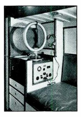
Two d-f installations on pleasure craft, both Bludworth models. The below-decks model (above) can be used inside wooden cabins. The model shown mounted on the cruiser (left) is completely water-proof and will operate readily when submerged in hot salt water
