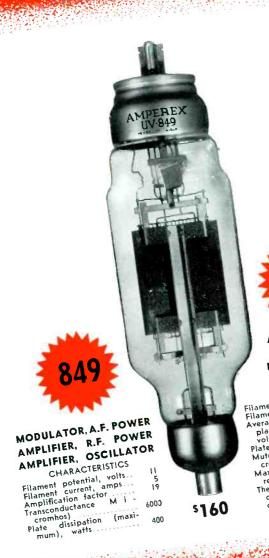
A.F. AMPLIFIER, MODULATOR R.F. OSCILLATOR, AMPLIFIER
