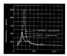
Fig. 10—Electrical impedance of loudspeaker in cabinet illustrating damping action of labyrinth
