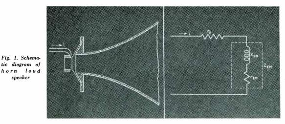
Fig. 2. Impedance presented to an electric current by horn loud speaker
