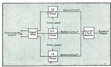
The auto-alarm receiver controls a relay which closes on each signal received. Three timers time the length of each signal and each space. If the signal is between 3.5 and 4.5 seconds long, and if the space is not longer than 1.5 seconds, a "count" is registered. Four counts actuate the alarm hells
