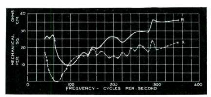
Fig. 8—Acoustic impedance of absorbent labyrinth measured at loudspeaker opening
