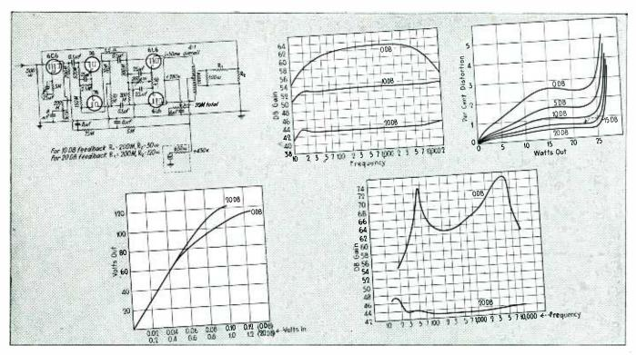
Figs. 5 to 9—Push-pull 6L6 amplifier circuit, its measured frequency response, and distortionoutput characteristic. Below, overload characteristic and (right) frequency response with loudspeaker load
