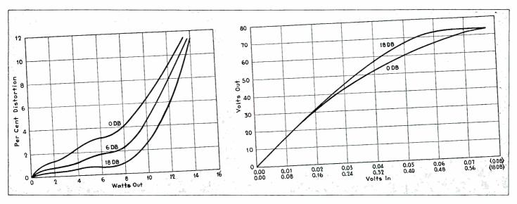
Figs. 12 and 13-Distortion and overload characteristics of the amplifier shown in Fig. 10. At 8 watts output, the distortion is halved by 6 db feedback, reduced below one per cent with 18 db feedback
