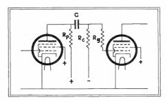
Fig. 1—Resistance coupled amplifier circuit for reducing the time of blocking when a large voltage impulse is applied
