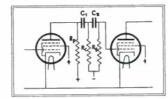
Fig. 2—By adding an additional blocking condenser and grid resistor, ordinary commercial condensers may be used in a stable resistance coupled amplifier
