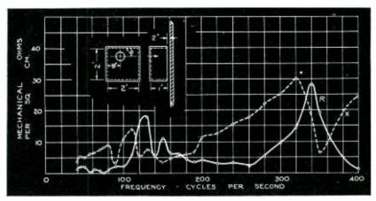
Fig. 7—Acoustic impedance of loudspeaker cabinet through 7-5/8 in.
