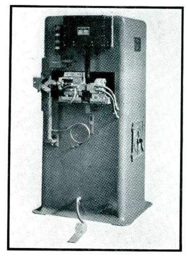
Early phototube temperature control unit for automatic heat treating valve stem tips; combines economy and speed
