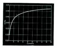
Fig. 3—Voltage output vs. illumination, high levels
