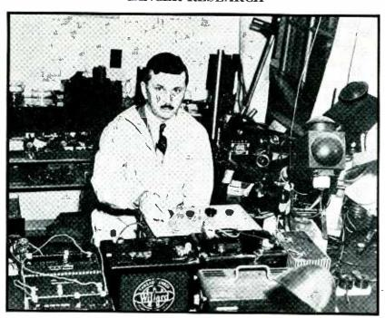
Professor Harold S. Burr, of Yale, with the vacuum tube microvoltmeter used for measuring the voltages produced in dying cell tissue. The high sensitivity, 5 microvolts, makes possible advance diagnosis of cancer
