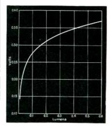
Fig. 4—Voltage output at low light levels
