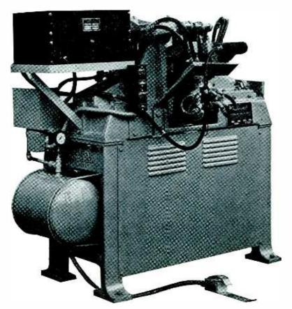
Heater for annealing central portion of the front axle king pin of automobiles; phototube control connected with amplifier by low capacity cable
