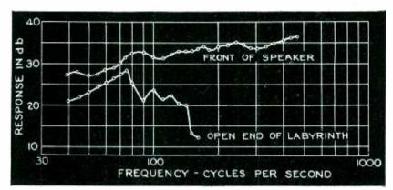
Fig. 3—Close-up response from front of speaker and from terminal opening of labyrinth
