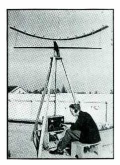
Parabolic reflector antenna used for receiving 1.5 meter signals from a stratosphere explorer balloon. At receiver is Prof. Easton of Caltech
