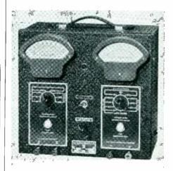
values from 250 micromicrofarads to 16 microfarads. The resistance ranges are from 2 ohm to 20 megohms. Operation of this unit is entirely from a built-in power supply. The unit, known as the Model 95 Super Unimeter, is offered in both portable and 19-in. relay rack mounting types.
