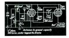
Fig. 2—Relay circuit using metal tubes
