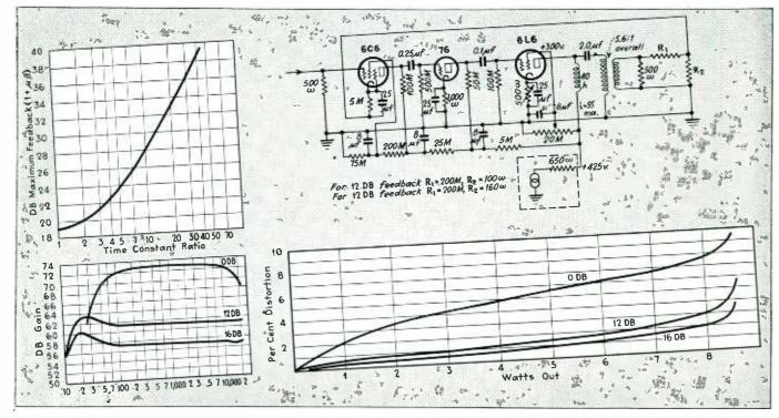
Fig. 1—(upper left) Maximum usable feedback in 3-stage amplifier with resistive feedback and usual coupling circuits. Figs. 2, 3, 4—Single-sided 6L6 unit, its measured frequency response, and single-frequency amplitude distortion vs. output power
