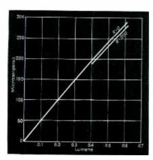
Fig. 1—Current output vs. illumination for low light levels
