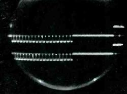
(4) Odd and even framing pedestals and sync. impulses
