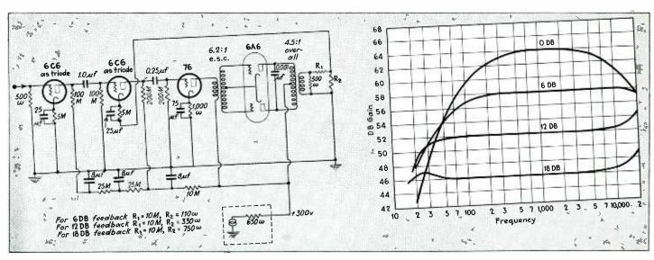
Figs. 10 and 11—A push-pull Class·B unit using a 6A6 double triode, with feedback applied over three stages. The measured frequency response (right) improves greatly as the feedback is increased
