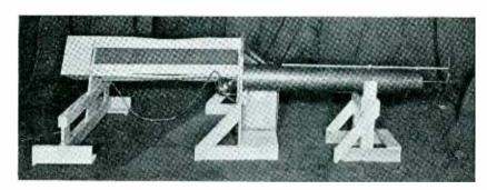
Fig. 5-Apparatus for the measurement of acoustic impedance
