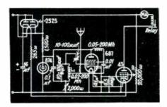
Fig. 1—Voltage-regulated relay circuit
