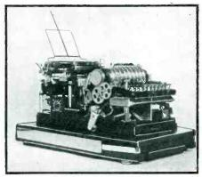
A new self-coding typewriter, electrically operated, is operated like an ordinary typewriter but turns out coded copy. Over 10 million code combinations are available in the device
