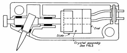
Fig. 4—Cross section of record-saving pickup
