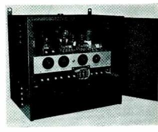
Amplifier cabinet used with the self-contained photo-relay
