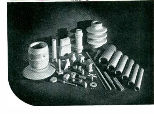
square inch, and specific gravity of 2.77. The dielectric constant varies from 5.76 at 60 cycles to 6.4 in the range 853 to 890 kc. The loss factor is about the same as the other clay-body porcelains. This particular ceramic is widely used in ignition spark-plugs.
