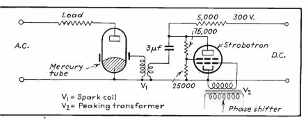
Circuit showing the use of a Strobotron for starting a mercury Fig. 6 pool rectifier used in a half-cycle welding circuit
