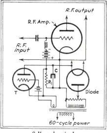
Self-synchronized diode circuit
