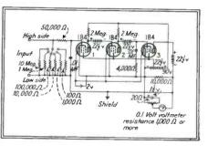
Schematic wiring diagram for instrument measuring 10<sup>-3</sup> to 10<sup>-8</sup> ampere, full scale
