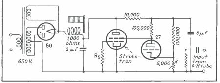
Fig. 4 Circuit diagram for a circuit to operate a message counter register for recording cosmic rays by a Geiger-Muller tube
