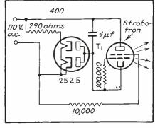
Fig. 3 Diagram of a 60-cycle stroboscope used at M.I.T.
