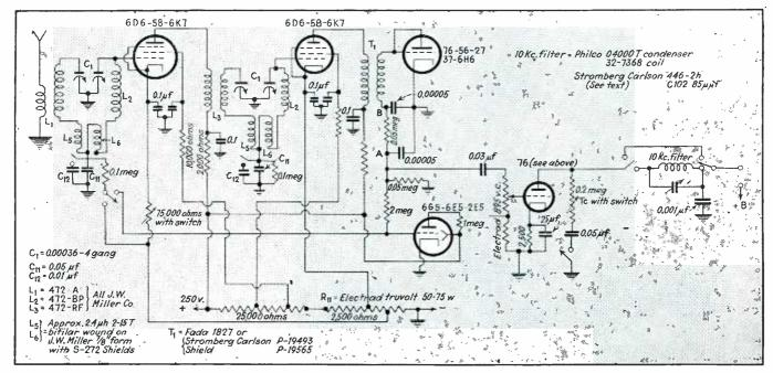
Circuit diagram, r.f. to output of first a.f. This tuner employs the selective circuits used in the well known Western Electric 10A receiver
