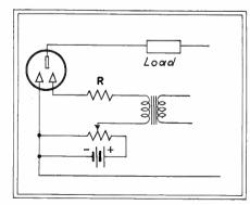
Relay circuit using new tube
