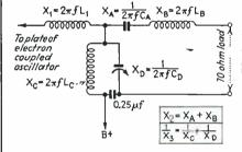
Fig. 3—Oscillator plate to line transformer
