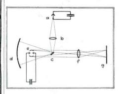
Diagram of the Schlieren method of photographing sound applied to a spark discharge
