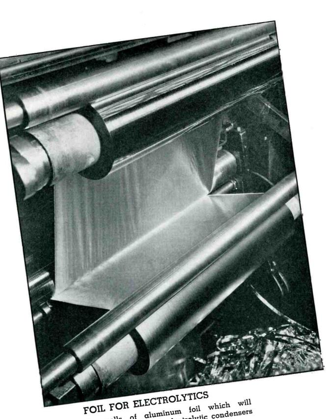
Side-trimming rolls of aluminum foil which will eventually serve as anodes in electrolytic condensers
