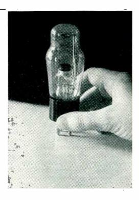
easier to start; that is, it requires a lower starting voltage on this grid to initiate the main discharge. The inner grid may also be treated in other ways to reduce the breakdown voltage and thus assist in starting the tube. The outer grid in the tube shown is of graphite, and it effectively shields the cathode and inner grid from the anode. Graphite has been used, since the breakdown voltage between it and the anode is not seriously reduced by condensed or
