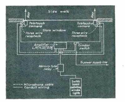
Set-up of Teletouch Ray for automatic window-lighting control
