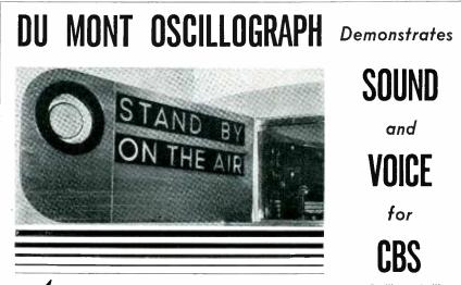
NOTHER of the unique applications of a Du Mont Cathode Ray Oscillograph illustrated here was conceived by Columbia Broadcasting System. On either side of Oscillograph employing a nine-inch Du Mont Cathode Ray Tube is mounted in the wall. These instruments are connected to the stage microphones and show the audience what sound and voice looks like. This application although interesting does not begin to show the usefulness of this fine instrument.
