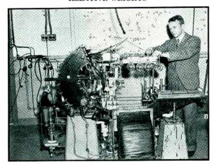
This new mass spectrograph at Harvard University treats streams of charged atoms like cathode rays, weighs them relatively, makes discovery of isotopes easy. Professor Kenneth Bainbridge is in charge
