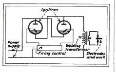
Two ignitrons connected for welding operation
