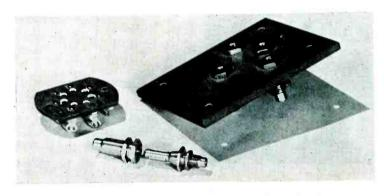
Mycalex (lead-less variety) machined into tube and coil-socket forms
