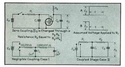
Fig. 5-Coupled and uncoupled two-stage filters
