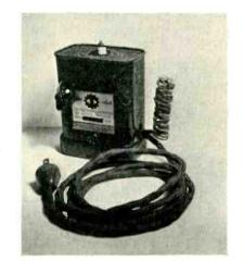
single-pole, double-throw type with silver-alloy contacts of 100 watts capacity. Relay sensitivity is controlled by a small bakelite knob on the side of the case. In operation, the antenna is connected to an insulated terminal at the top of the case. The relay may be used in a number of applications such as counting metallic objects, control of certain industrial operations, animated advertising displays, opening doors, etc. The \$25.00 complete. The CR-1 relay lists at
