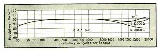
Fig. 6—Typical calibration curves at 100% modulation, 1 ma. direct current, and various values of circuit resistance
