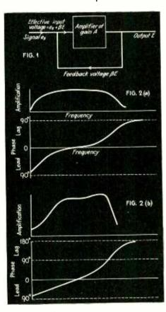
Fig. 1.—Fundamental feedback circuit, showing relation between input, output and feedback voltages
