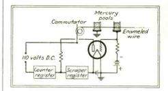
Circuit for testing enamel wire
