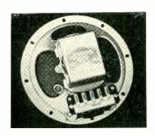
impedance values and the other to match conventional line impedance values. The illustration shows a speaker for plate impedance matching suitable for impedances of 4,500, 7,000, 10,000, and 14,000 ohms. Besides a full line of speakers with adjustable impedance transformers, the speakers and impedance matching transformers may be obtained separately from Jensen.
