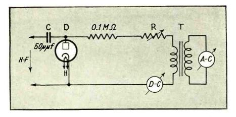
Fig. 1-Fundamental schematic wiring diagram for modulation meter
