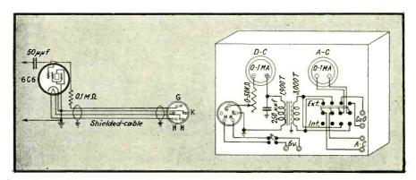
Fig. 3--Schematic wiring diagram and layout of the complete meter. The tube is connected through the shielded cable to the measuring circuit
