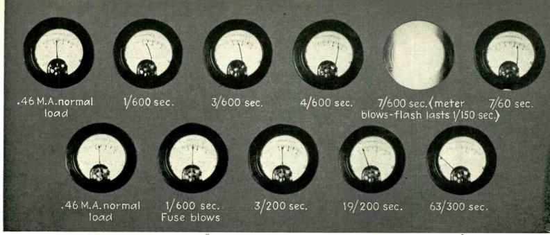
Top line—Milliammeter (0-1) subjected to direct short circuit across 110 volts. Bottom—Effect of fuse in protecting meter against direct overload
