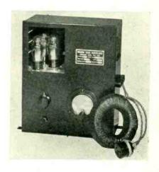
meter shunted across the condenser to determine the condenser charge. The instrument has three ranges, obtained by shunting the transformer secondary by resistors of different values. The instrument is calibrated in r.m.s. values of current. In operation the primary lead to the electric welder is passed through the doughnut shaped coil which forms the current transformer.
