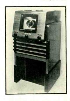
This Telefunken receiver, ready for the market, has a 20,000 volt cathode ray tube behind the lens, through which the image is projected
