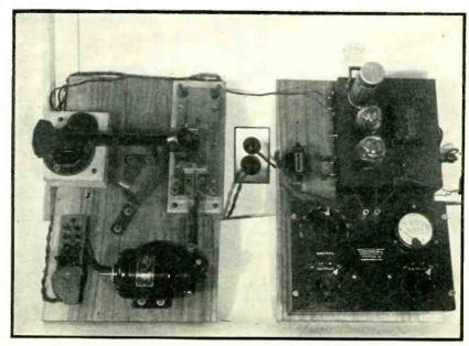
Fig. 1. Pick-up surface tester and amplifier
