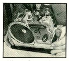
This carrier telephone unit for interoffice use sends r-f energy over the power line. The dynamic speaker serves as speaker and microphone
