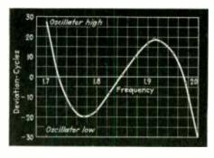
Fig. 2—Graph showing deviation from perfect tracking
