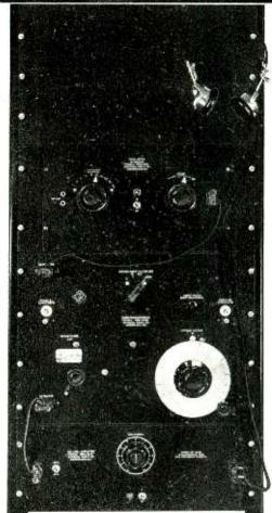
TILE assembly above is completely a-c operated. It is composed of the Type 508-A Oscillator (top), Type 716-A Capacitance Bridge, Type 714-A Amplifier and Type 480-B relay rack. Price, complete with bench-mounting relay rack (without headset), \$660.00
