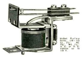
Air gap control permits quick adjustment to varying requirements during assembly even though the machines are built to identical specifications. Mounting is designed for production line requirements; consists of a single 8/32 screw and shake-proof washer with locating pin that prevents loosening or turning.
