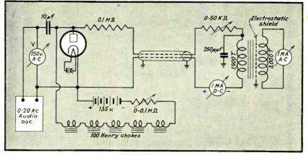
Fig. 4—Circuit arrangement for making accurate meter calibrations
