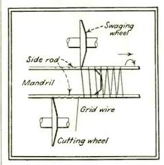
Fig. 2—Details of grid winding machine
