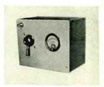
wire. If a person or car approaches within 3 ft. of the antenna the device operates closing a relay for operating any desired device. The device is useful where photo-electric apparatus or the installation of "Treads" is not possible. The complete unit less antenna lists for \$40. The size of the box is  $6\frac{1}{2} \times 8 \times 5\frac{1}{2}$  in. overall.
