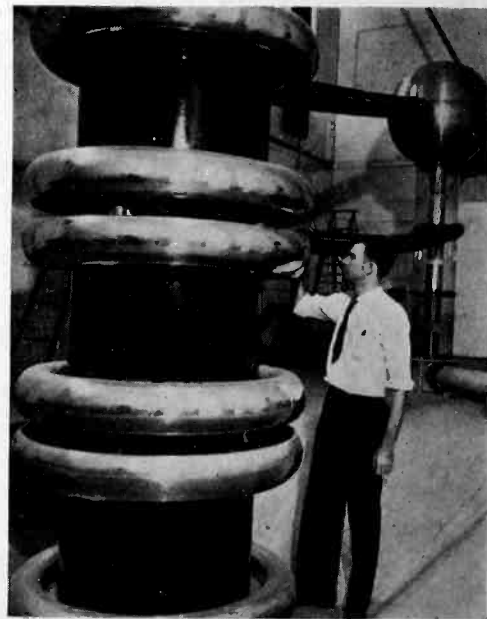
This 17-foot monster is a deuteron bombarder, recently constructed at the University of Michigan. It may be used either for producing artificial radioactivity or x-rays of one million volt energy
