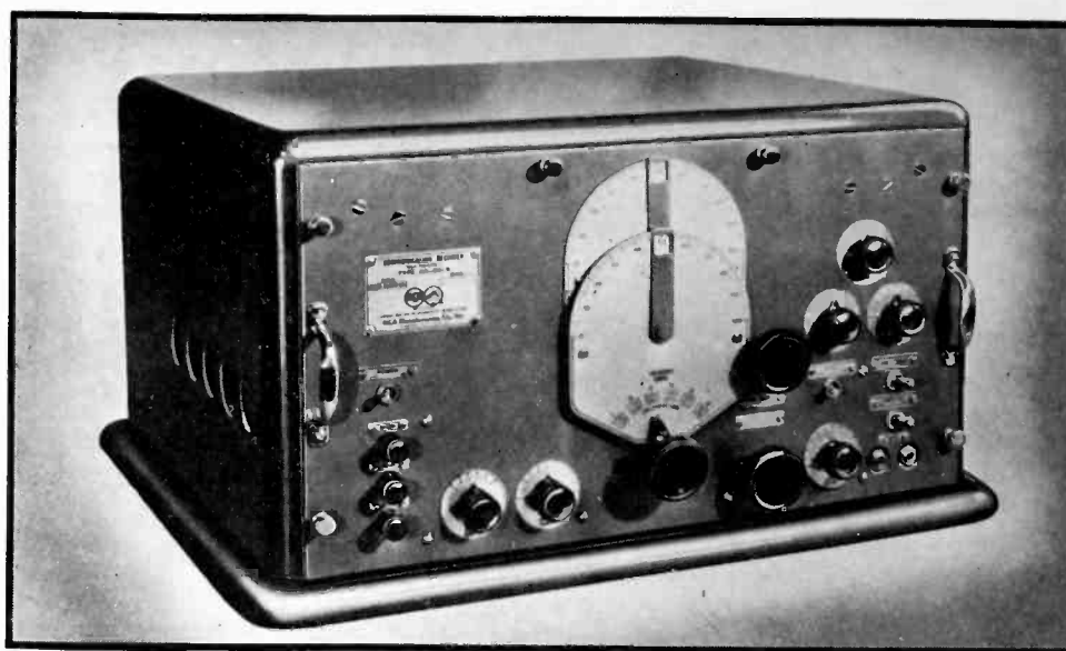
The AR-60 of RCA, with main and band spread tuning dial of unusual construction
