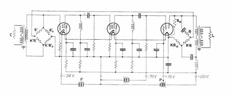
Above, representative amplifier circuit, with bridge-type feed-back
