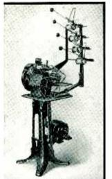
**Control of every variable** in the winding insures production of coils identical in electrical characteristics. Tension, pressure and wire spacing are determined by positive adjustments. Length of winding is determined by accurately cut cams. The new, quick-setting counter automatically stops the machine when required turns are wound. Actual plant records show gains of from three to four times the production of a single-coil winder.
