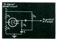
Static limiter circuit, described in the text (G. E.)
