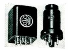
tubes. These units are claimed to have a response plus or minus 2 db. from 30 cycles to 20,000 cycles. They measure  $1.7/16 \ge 1.7/16 \ge 1.5/16$  in., having an average weight of  $6\frac{1}{2}$  oz. They are intended primarily for noise meter, aircraft and remote pick-up work.
