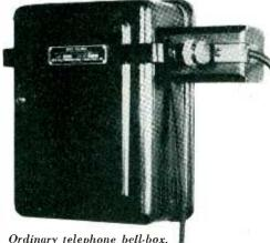
Ordinary telephone bell-box, showing method of coupling to put facsimilie signals on the line
