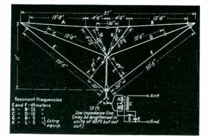
Spiderweb all-wave antenna developed by RCA engineers
