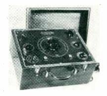
ray tube, a 6J7 is used in the dual frequency oscillator and an 84 for rectifying. The ranges are 2 mmf. to 100 mmf. in capacity, less than one ohm to one megohm in resistance, and from 10 microhenries to 100 henries of inductance. The visual indicator is also available as a null indicator for separate A-C bridges. In this form the tube is combined with a 79 as a two-stage resistance coupled amplifier. When so used the indicator is substituted directly for the usual telephone receivers.
