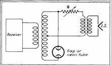
In this patent a circuit is shown involving an output transformer connecting the receiver to a loud speaker. A neon tube is substituted for the gap shown in the original patent and at a certain value of resistance, distinct noise limiting action occurs.
