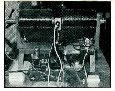
Chamber unit with Geiger counter mounted in an electromagnetic field for reflection of Alpha particles
