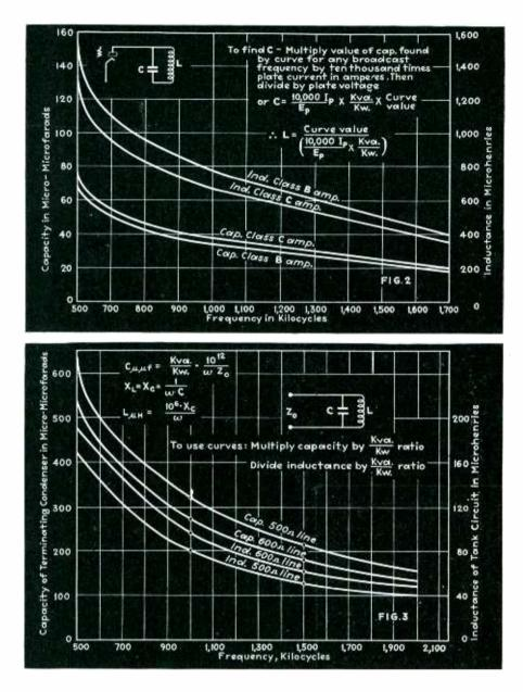
**283** Charts for calculating capacity and inductance of radio-frequency amplifier tank circuits
