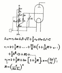
tively coupled with each other, the selfinduction value (L12) of the coupling induction of the separate members of the wave-band filter substantially answering to the equation for  $L_{12}$  as shown on the illustration wherein  $L_1$ is the constant self-induction, C the variable capacity of the separate sections of the filter and  $\tau_1$  and  $\tau_2$  are determined by the equation shown on the figure where R is the resistance of the separate sections of the waveband filter.
