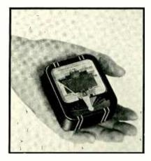
illumination levels are fully and legibly indicated. The scale is divided into five "seeing task" zones, set off by colored divisions. The back of the indicator contains an embossed metal plate classifying specific seeing tasks so completely that no assumptions need be made by the user.
