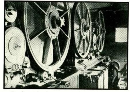
This self-contained steel-tape magnetic recorder, installed in a truck, is used in Berlin to gather opinions from the man in the street, news events, etc., which are later broadcast in an evening program called "The Echo of the Day"
