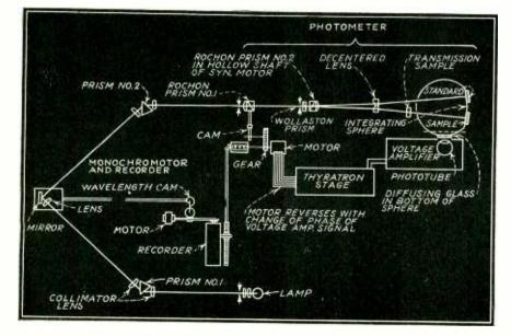
Schematic diagram of the automatic recording color analyzer, described in the text
