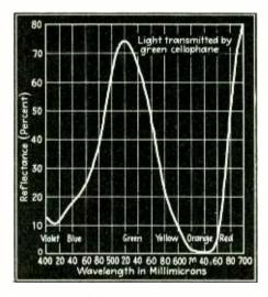
A typical record produced by the color analyzer (the transmission properties of green cellophane)
