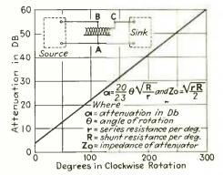
To accomplish this attenuation a variable ladder network consisting of a series element on which the contact rids, and which has a shunt element connected to it along its entire length, is used.
