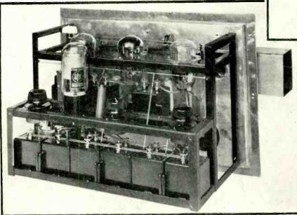
Interior of an intermediate amplifier showing low loss construction and the use of a neon stabilizing device. The amplifier boxes are double screened and sound proof
