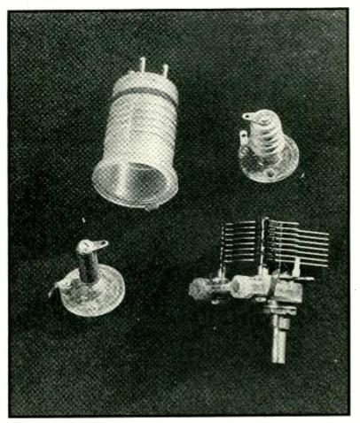
Na-Ald parts of low power factor made from Victron or imported poly-styrol. R-f chokes, a coil form, a variable condenser
