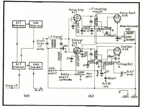
Fig. 1. Block diagram (a) of the noise-silencing circuit, and the complete connection diagram (b)
