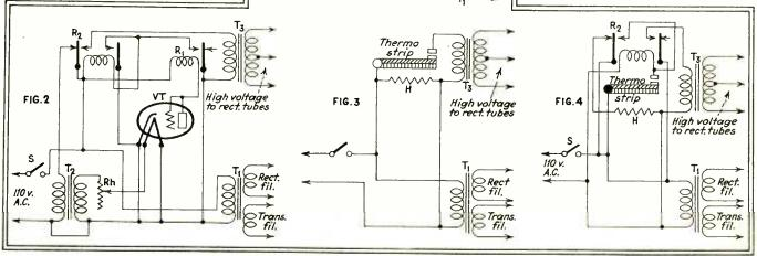
Circuits for introducing a time-delay in the application of high voltage to the plates of mercury-type rectifier tubes
