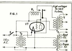
If, during the operation of a transmitter, S is opened and closed again quickly, the time-delay tube, having cooled in the meantime, would have to heat all over again before plate voltage would be impressed on the rectifier tubes. The only possible failure of the time-delay equipment to work with this circuit would be in the event that the line switch was opened and quickly closed in the five or ten seconds before the time-delay tube had a chance to cool after the actuating of the R2 relay.
