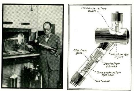
Arturo Castellani with his télépantoscope, a cathode ray television scanner similar to those developed in this country by Zworykin and Farnsworth. Italian television experiments by the Safer Company in Milan have made use of a 500 watt, 7 meter image transmitter in conjunction with a 50 watt, 5 meter sound transmitter. A receiver (240 lines 25 frames per second) is available for approximately 640 dollars
