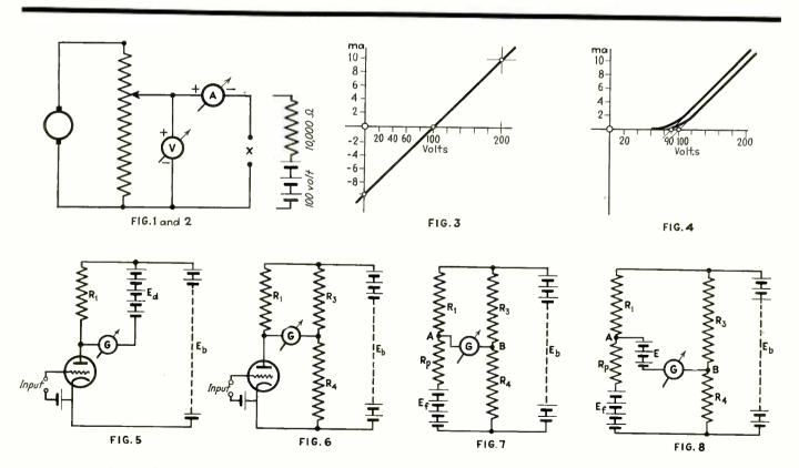
Given a box with two terminals, an engineer would determine its E-I characteristic as in Figs. 1-3 deciding that Fig. 3 represented Fig. 1 and 2. But given Fig. 4, the problem would not be so simple. Mr. Richter shows how the plate circuit theorum can be applied practically to a bridge circuit with a vacuum tube in one arm—or to other circuits
