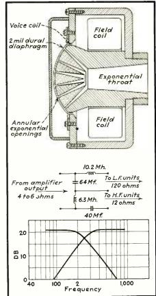
High frequency unit (Lansing) and series-type dividing network
