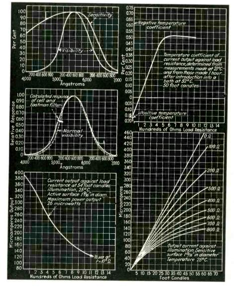
Quantitative data on the G. E. Blocking Layer selenium-platinum selfgenerating photocell
