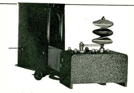
An early model of a 90 line mirror screw receiver made by TeKaDe, showing the Kerr Cell container and cylindrical lens
