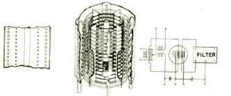
and in line with them. A metal shield surrounds the whole. The method of support shown is not material: each anode is supported by a pair of metal posts cut away to clear the other anode; and the grids are supported from the anodes by mica spacers.
