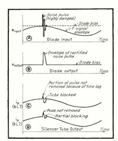
Fig. 2—(A) Diode input of signal envelope (only one edge shown) and noise. (B) Rectified envelope of noise peak applied to blocking grid of silencer. (C) Effect of blocking action on i-f envelope.
