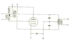
Fig. 8. Circuit with deflection tube similar to a conventional triode
