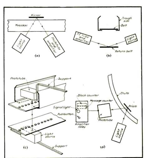
A and B—Light beams are projected through a belt—or across its surface. C—If the rate at which beam is interrupted decreases, an alarm sounds. D—How the phototube measures the ratio between messages successfully transmitted to those that stuck temporarily
