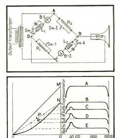
Above, the bulb-expander circuit and below, the expansion and bassboosting characteristics
