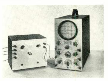
Another feature, contributing to outstanding performance is an *Improved Synchronizing Circuit* permitting locking sweep with fractions as well as multiples of wave.
