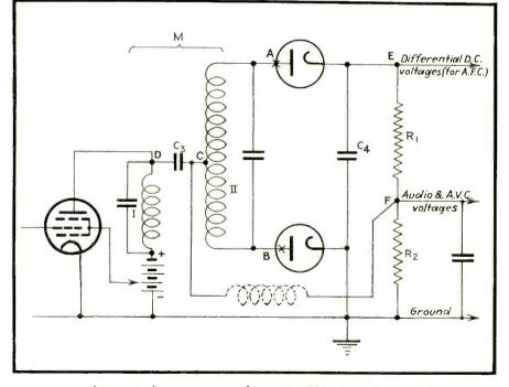
Automatic frequency control circuit. The choke is optional
