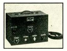
output of the oscillator is connected to the input of the model 81 whose frequency modulated output is in turn connected to the receiver under test. This eliminates the necessity of installing a jack or other alterations which may destroy the instrument's accuracy of calibration. Net price of this device complete with tubes and built-in sweep motor is \$34.25.
