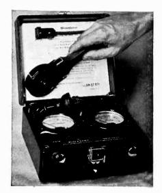
meter-ammeter with cable extensions, switches and plugs for illumination engineers who wish to analyze voltage and current in addition to light intensity and distribution.
