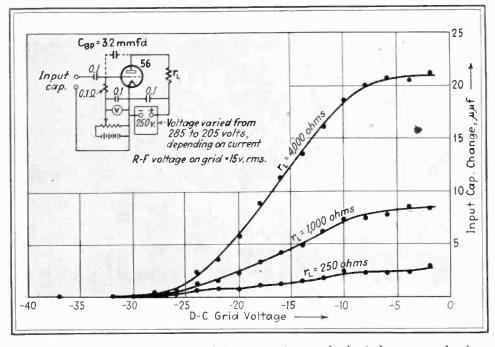
Extent of capacity change secured from use of a standard triode as control tube
