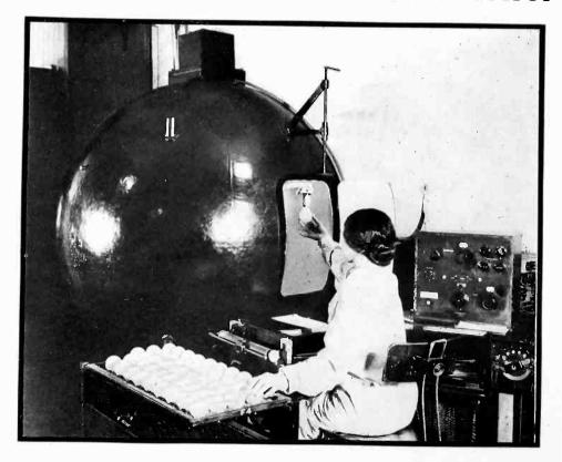
This integrating sphere directs the entire light output of a sample lamp, taken from the production line, into a photocell mounted on top, which in turn measures the light output in lumens
