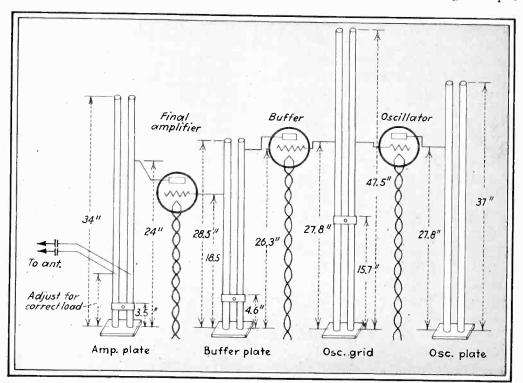
The mechanical layout of the transmitter showing dimensions of resonant lines, position of shorting bars and connections to the plate and grid circuits. Type 45 tubes are used throughout
