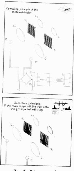
How the Petoscope works
