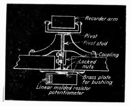
, Mechanical coupling of {recorder arm to resistor
