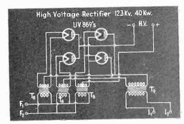
High voltage power supply for h-f generator
