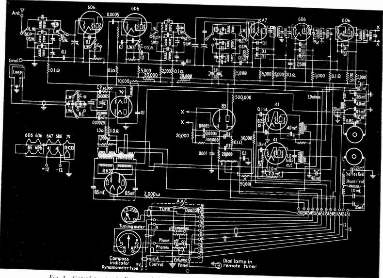
Fig. 3. Complete circuit diagram of the Lear Developments Co. dynamometer type radio compass.
