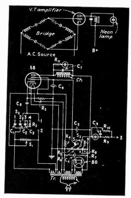
Fig. 1. (A) Above, fundamental circuit (B) Below, complete diagram of analyzer
