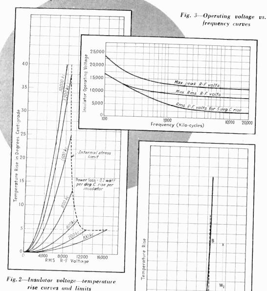
An interesting analogy also exists between the behavior of a solid dielectric and that of a material like steel under mechanical stress. The strain is proportional to stress up to the elastic limit, beyond which the steel receives a permanent set. If the stress is increased much further, the material eventually breaks; if the stress is removed before failure occurs, the specimen may later be subjected to lower stress with only slightly different characteristics.
