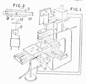
intensity and thereby of the output current. For example, a replica in paraffin wax, celluloid, gelatine, or other translucent material is used for modulating the light intensity for controlling a cutting machine to reproduce a three-dimensional object. J. Dorn, C. E. Duits and A. Gore. No. 424,802.
