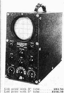
• BASICAL-LY NEW SWEEP having a range from 10 to 100,-000 cycles per second with improved linearity and exceptionally fast return trace.
