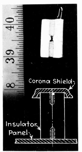
Fig. 1—Below, outline of typical insulator. Above, insulator after breakdown (actual size).
