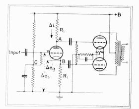
Mr. Richter's circuit for coupling a driver to a push-pull stage by a capacity-resistance network
