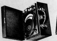
Model 310 DC and Single Phase AC Wattmeters
