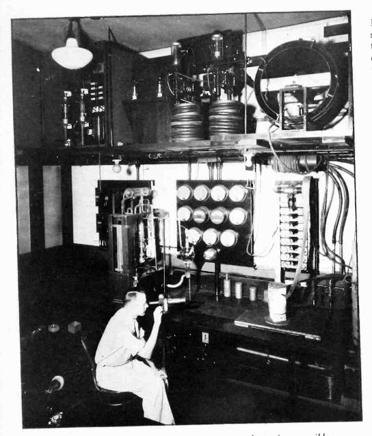
The high frequency generator used to heat a charge in a crucible, in the Westinghouse Laboratories. The output transformer is shown at the upper right, with the amplifier tubes to the left
