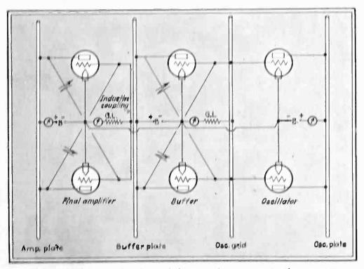
Each varied bar in the closified diagram above represents the resonantline infolded, i.e., the center of each is the shorting bar. The neutralising condensars consect directly from plate to grid in each case
