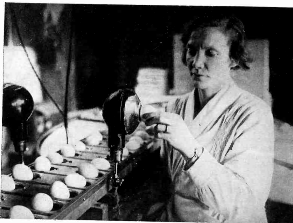
In Warwickshire, England, 50,000 eggs per week are tested for edible qualities by phototubes
