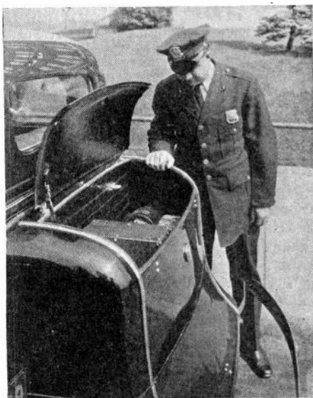
The power supply of this ultra-short wave patrol car transmitter is placed in the rear trunk, an unobtrusive but easily accessible location.
