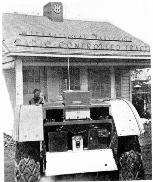
The International Harvester Company is exhibiting this remote-controlled tractor, which plows acreage while steered from the farmhouse porch.
