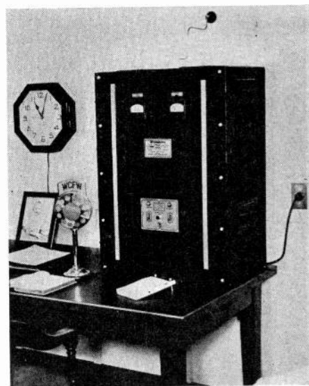
A medium wave transmitter of modern design. Note the simplicity of connections to power supply, microphone and antenna.
