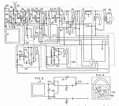
Patent granted to Bendix Aviation Corporation for an installation to be used (a) for direction finding on ordinary broadcast transmission, when the effect of modulation on a visual type of indicator is eliminated by a local heterodyne, or (b) as a non-directional receiver for reproducing programs. British patent No. 404,659.
