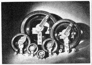
Ohmite all-porcelain vitreous enameled rheostats are now made in six sizes from 25 watts through 500 watts to satisfy almost any rheostat need. Because of their unique construction each turn of wire acts as a separate step and extremely close control is obtained.
