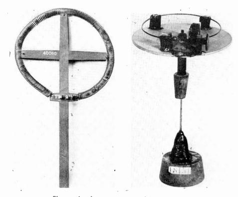
Photographs of two resonators used by Heinrich Hertz in his demonstration of the existence of electric waves
