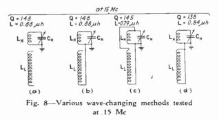
Popular methods of band switching affect Q of the highest frequency coil to practically the same extent. A choice between methods should be based on other considerations, one being the performance of the lowest frequency coil.
