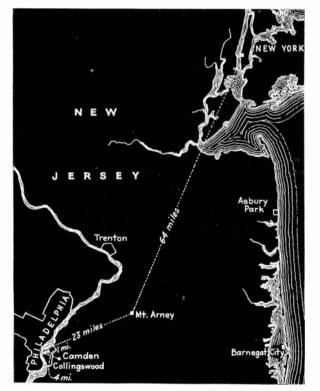
Path of 49-50 megacycle waves from New York to Camden which underwent one radio relay enroute to be rebroadcast and "seen" at Collingswood
