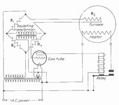
Fig. 1—Bridge circuit in which one arm is a resistance thermometer
