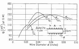
Fig. 2-Effect of changing wire diameter
