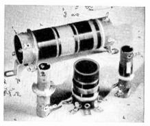
(Above) Coils protected with Bakelite Varnish, and (left) Bakelite Laminated terminal strips and discs all used in Pilot All-Wave Receivers,
