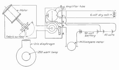
Arrangement of apparatus for measuring luster or sheen of fabrics on face of pulley. Photocell indicates reflection from textile
