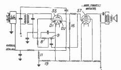
is made inoperative under the control of a diode detector when the input energy is below a predetermined level. W. A. Harris, Marconi Co. No. 404,583.
