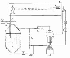
Fig. 3-System used in growing crystals
