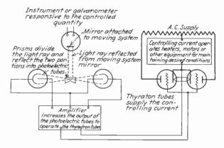
Fig. 5—Precision control circuit that maintains temperature to within 0.005 deg. C.
