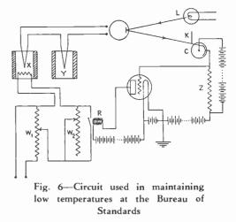
power without batteries using only one slide-wire rheostat with four sliding contacts to furnish all the sources of potential for the phototube and its amplifier.
