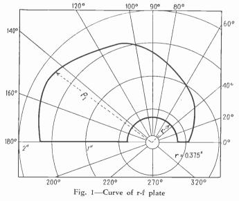
tion for determining the physical dimensions of the curve of condenser plates, without resorting to graphical solutions. It is divided into two parts. In Part I, is presented the exact solution for determining the physical dimensions of the curve of the oscillator section necessary for single dial control when the physical and electrical constants of the radio frequency tuning section are known. Part II is concerned with the use of the
