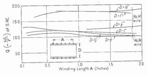
Fig. 5-Relation between winding length and Q
