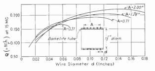
Fig. 4-Effect of wire diameter on large coil
