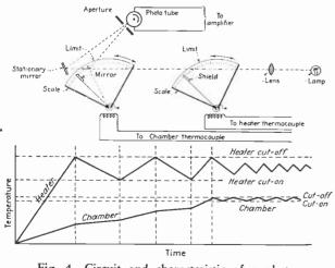
Fig. 4—Circuit and characteristic of a phototube method of maintaining temperature
