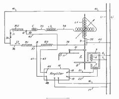
Rotating machine control. A dynamo and a circuit including a battery and a substantially constant load, such as saturated tubes, and a means for controlling the field strength of the machine. G. J. Hausamann, Eclipse Aviation Corp. No. 1,958,665.
