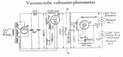
Circuit described by Mr. Fink consisting of a source of constant voltage, balanced photocell input to vacuum-tube voltmeter
