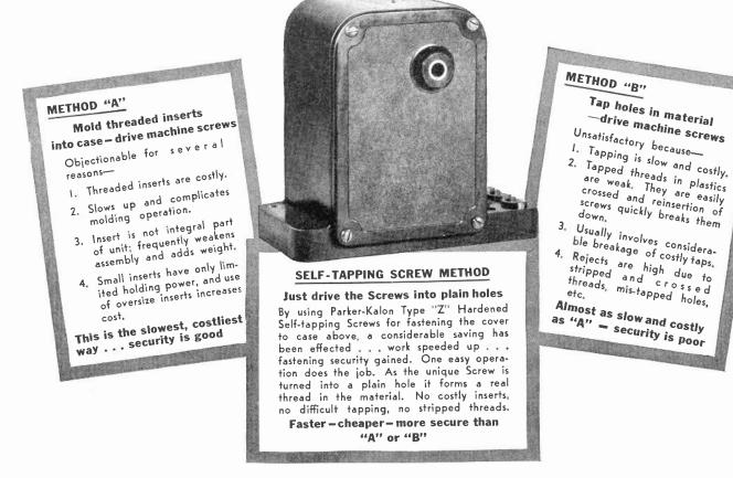
It is easy to see why scores of manufacturers recognize Self - tapping Screws as the fastest, cheapest, strongest means of making most fastenings to plastics.
