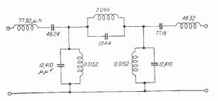
Fig. 2—Schematic of a high frequency filter designed by methods employed at low frequencies.
