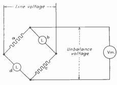
Fig. 1—Bridge circuit composed of resistances and lamps
