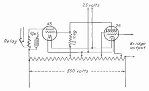
Fig. 4-Elementary diagram of voltage relay
