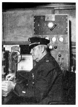
Officer in charge of Hoboken, N. J., 8-meter, two-way system (REL) converses with mobile force
