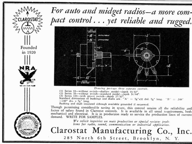
For auto and midget radios—a more compact control ... yet reliable and rugged.
