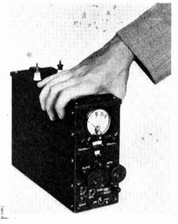
Compact 5-meter receiver-transmitter (RCA) for portable use
