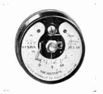
The relay will make contact on values down to three microamperes or one millivolt and its contacts are capable of handling five watts at 110 volts.
