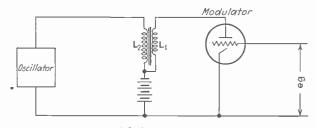
Fig. 3-Modified constant current system
