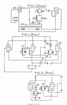
**Phase modulation.** Two components of the same carrier wave phase displaced by 90 deg. are radiated simultaneously from separate aerials after being modulated by signal currents in phase opposition. For reception it is necessary to supply a local oscillation of the same frequency, but de-phased from the incoming carrier so that the signals cause minimum interference with any normal type of receiver. G. W. Walton, London. No. 400,273.
