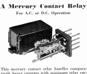
tively heavy currents with minimum relay current consumption. It is quick-acting, nonchattering, and can be equipped with one or two mercury contacts, easily adjustable for either make or break operation. Supplied either with angle bracket or on Bakelite base with cover, and for a variety of voltages and frequencies. (D.C. relay shown in illustration.)
