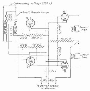
Fig. 6-Double-acting electronic voltage relay
