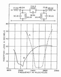
Fig. 4—(left) Modification of L and C of Fig. 2, so that the resonance frequencies are the same as before, changes the characteristics of the filter from A to B.
