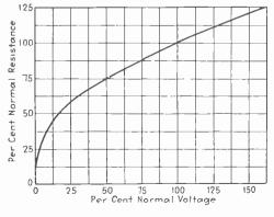
Fig. 2—Voltage-resistance curve—25 watt tungsten lamps
