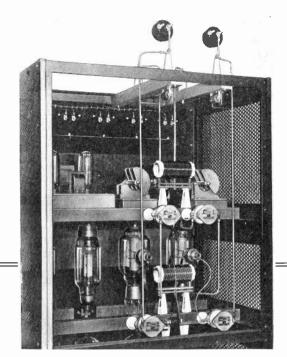
Admiral Byrd's Antarctic transmitter built by Collins Radio
