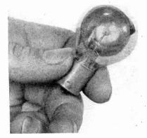
known as the FJ-114 is made in an automobile headlamp bulb and therefore is much smaller than the average tube. The active surface is caesium deposited on oxidized silver, enhanced by other special treatments which not only contribute to the high sensitivity (35 microamperes per lumen) but produces a high sensitivity in the infra-red.
