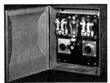
adjustable from 1/10 second to 45 seconds. It can be applied to any spot or projection welding machine now in service which is equipped with a magnetic main contactor. The electronic timer is unusually rugged, as the industrial grid glow tube is designed for sturdiness and long life and operates the contactor directly without delicate intermediate relays. The grid glow tube is free from any effects of wide temperature changes.
