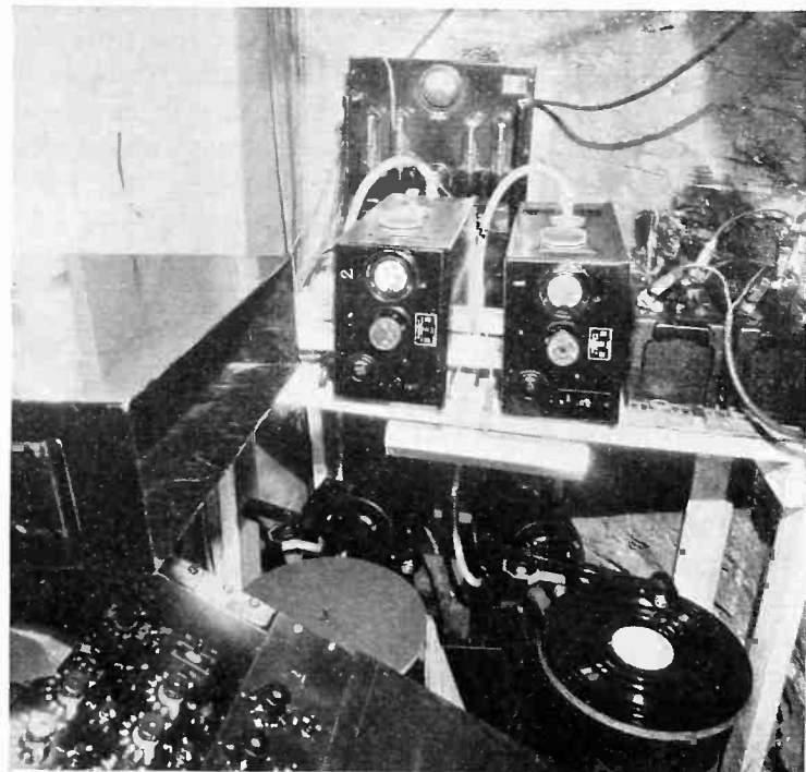
Transcriptions and amplifier outfits used to provide background sounds in stage productions. Mob-scenes, storms, wind effects, choruses, "ghosts," etc., can be presented in this way
