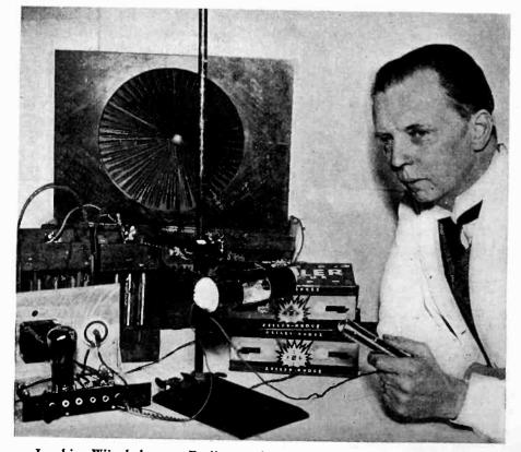
Joachim Winckelmann, Berlin, sends a continuous current through a selenium cell; when light falls on the cell a tone emitted by an oscillator varies in frequency with the intensity of illumination
