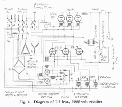
This type of rectifier is suitable for applications above about 2,000 volts direct current as in such cases the cost of d.-c. generators rises rapidly. By proper choice of tube types d.-c. voltages up to 10,000 are obtainable.
