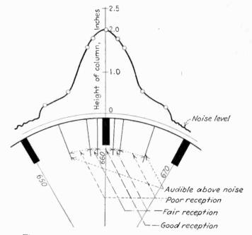
Fig. 3-Action of tuning-indicator on local signal
