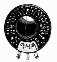
A  $2\frac{3}{4}$  in. circular refractory plate forms the base for the special resistance wire of low temperature coefficient of resistivity. The plate, wire, contacts and terminal connections are thoroughly protected against corrosion and damage by fused-on vitreous enamel.
