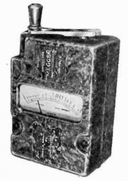
In common with other Megger instruments, the Midget tester consists of a true ohmmeter, direct-reading like a voltmeter, combined with a special d.c. hand generator. The scale reads as high as 20 megohms and the generator supplies testing current at 500 volts, thus obviating necessity for depending on batteries or any other outside source of current.—*Electronics*, *February*, 1933.
