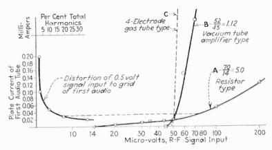
Fig. 6-Characteristics of three noise-gate systems
