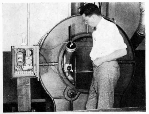
When coffee in this McCormick roaster reaches that particular shade of golden brown which indicates that the ideal roasting has been secured a Weston photoelectric cell notifies the supervisor to recharge the roaster
