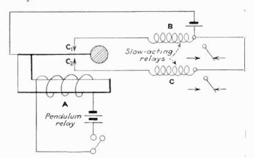
Fig. 2-Pendulum or vibrating reed relay
