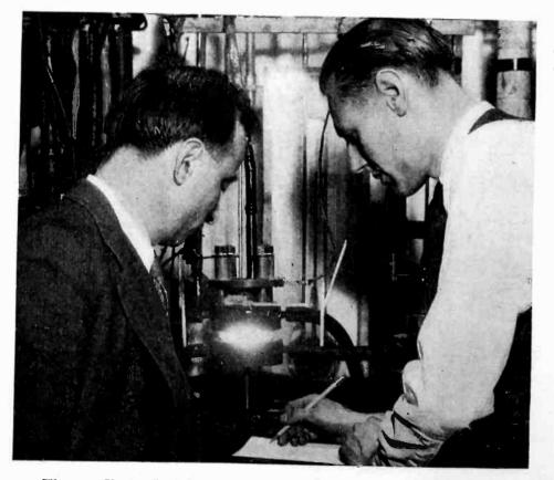
The new Slepian-Ludwig method of controlling a mercury arc by means of a high-resistance rod partly immersed in the mercury pool, was exhibited at the January convention, A. I. E. E.
