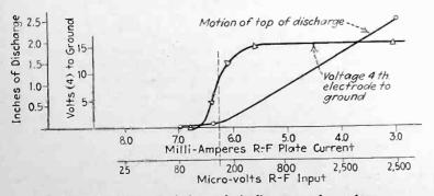
Fig. 5-Characteristics of indicator tube when adjusted to exclude signals below 200 microvolts
