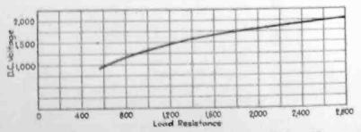
Fig. 2-Regulation curve for Thyratron-controlled rectifier
