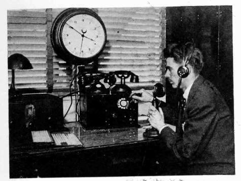
An "automatic dial" selects the wavelength wanted, in this new short-wave set used by the United Air Lines, Chicago. Any one of five or six planes can be reached by dialing its number
