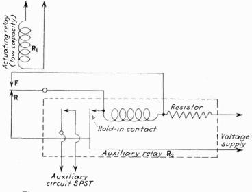
Fig. 3-Auxiliary relay circuit with lock-in feature
