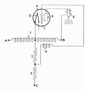
Fig. 1—Elementary diagram of the phase-failure relay
