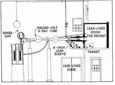
The great 900,000-volt X-ray tube of the Memorial Hospital, New York City. In this tube the electrons are twice accelerated before they strike the target, producing X-rays of tremendous penetrative power
