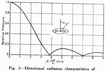
vibrating disc in infinite baffle
