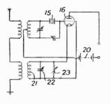
Coupling system. A coupling system operating over two distinct frequency bands, the required band being selected by the short-circuiting of one out of two or more transformer secondaries. W. A. MacDonald, assigned to Hazeltine Corp. No. 353,447.
