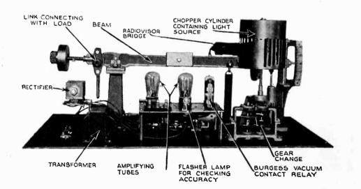
The telepoise with its light-sensitive selenium bridge which indicates the number of interruptions by the "chopper" cylinder
