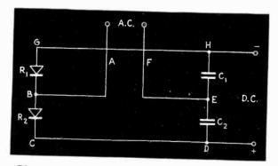
Fig. 1—Fundamental voltage doubler circuit
