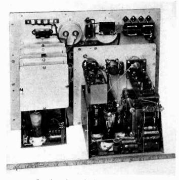
Interior of standard-signal generator with shield removed
