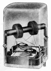
chassis, and held by two spade bolts. The coils are carried on a low-loss coil form and are extremely efficient in selectivity and gain. Compactly assembled, the coils are mounted on a newly developed material known as Learite and enclosed in a satin finished can.—Electronics, February, 1932.
