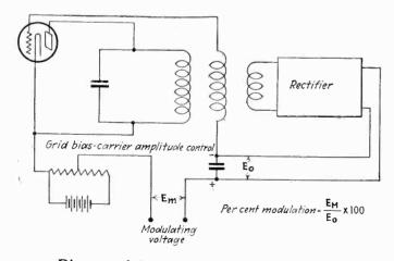
Diagram of Arguimbau method of obtaining constant output
