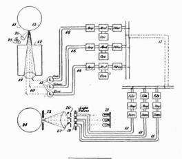
**Recording system.** A method of projecting a recording fluid toward a record surface, in accordance with the received signals. R. H. Ranger, assigned to RCA. No. 1,841,452.
