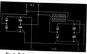
Fig. 3-Preliminary attempt to double the output voltage
