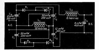
Fig. 5—Constants of the commercial voltagequadrupler
