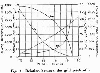
Fig. 3—Relation between the grid pitch of a triode and its characteristics
