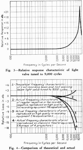
Fig. 4—Comparison of theoretical and actual losses in sound system
