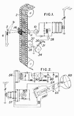
Glow lamp screen. Linear glow lamps which light up successively under control of voltages applied through timelag circuits. O. von Bronk, Berlin. No. 836,760.
