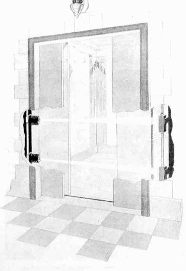
Phantom view of "electric-eye" and light projector for "Safe-T-Ray" equipment
