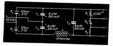
Fig. 2-Circuit constants of a modern commercial voltage-doubler
