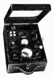
scale and to a resistance of 4,000 olims. The scale also carries indications in decibels, so that power level readings may be taken above or below the accepted value of zero level, 6 milliwatts in a 500 ohm load.
