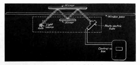
Moisture on the window pane interferes with light beam's passage to electric eye, controlling humidifier
