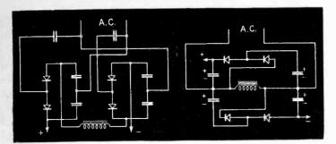
Fig. 4—Two circuits evolved in the development of a voltage-quadrupler
