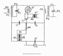
Cold cathode amplifier. Circuit which is described more fully under British patent granted to J. M. Schmierer, assigned to Radio Patents Corp. No. 1,838,871.
