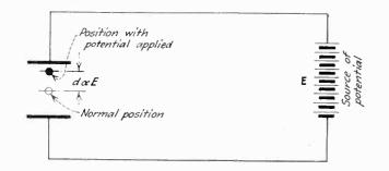
Fig. 1—Deflection is proportional to applied potential
