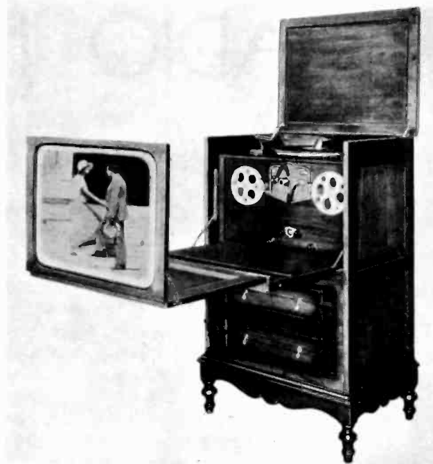
This complete cabinet model which includes radio and storage space for films was developed by the Talkiola Corporation
