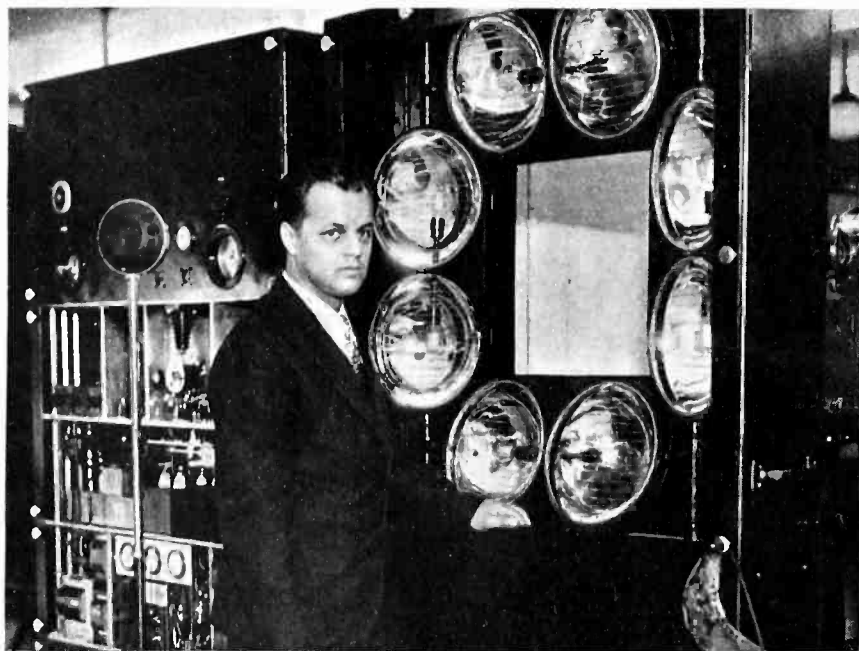
U. A. Sanabria with his latest type of television pickup which provides for picture transmission and reception on a six-foot screen
