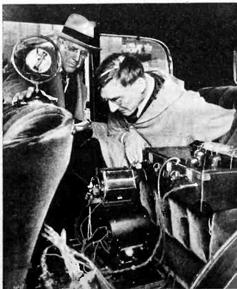
Dr. William Braid White making oscillograph records of noises inside a car, seeking a solution against obnoxious sounds
