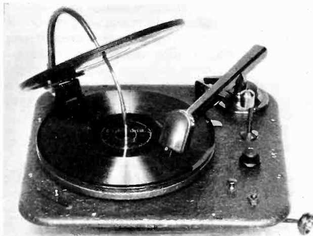
Record changer designed by Allen-Hough Carryola Company, handles up to ten records
