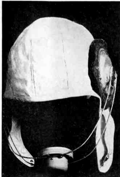
This combination receiving and sending headset used by Boeing pilots on their air-mail and passenger planes enables them to talk to ground stations 200 miles away.
