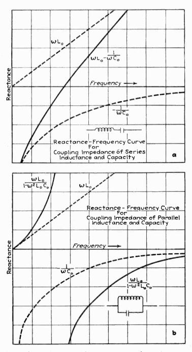
Fig. 2---Reactance-frequency curves for seriesand parallel-tuned circuits
