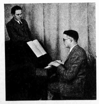
The photo-electric organ developed by Prof. A. C. Hardy of Cambridge, Mass., using tone-wheels on which vibration curves are photographed
