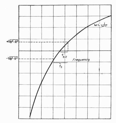
Fig. 5-Reactance-frequency curve of tuned circuit
