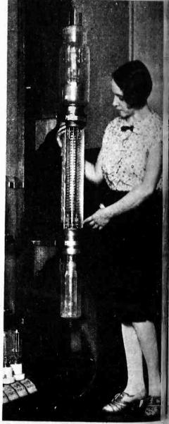
One of the 200-kw. tubes install in the new KDKA station, ne Saxenburg, Pa.
