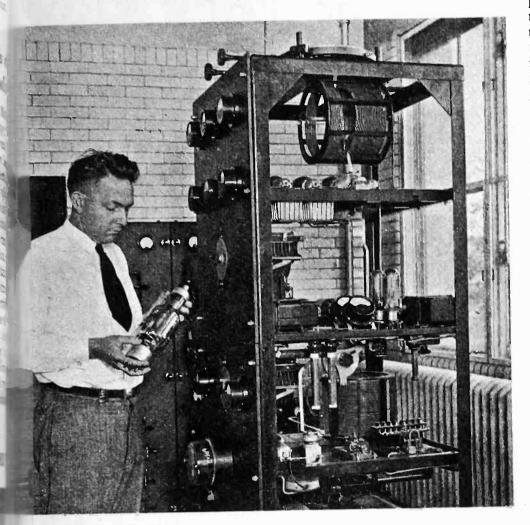
transmitter which broadcasts half-hourly weather reports from Station 'QDW, for the guidance of traffic on the airways radiating from Detroit. he operator is holding one of the ten 250-watt tubes with which the transmitter is equipped
