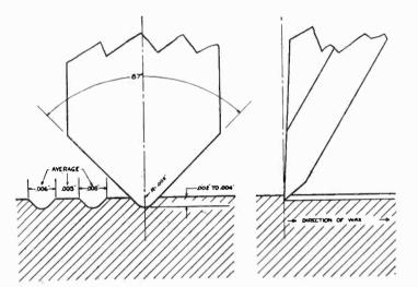
Fig. 1-Details of the stylus point of a wax cutter
