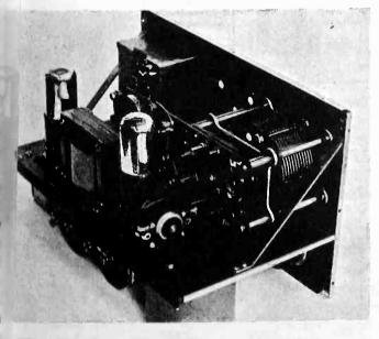
Interior of generator, using switching scheme of Fig. 3
