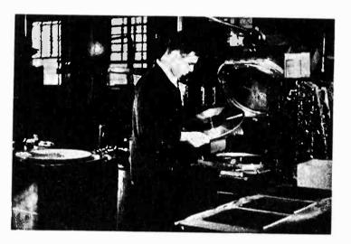
Fig. 2—Record press, showing finished record just removed from the dies, and record stock heating on the steam table
