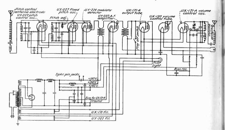
Circuits of the antenna-operated theremin. One antenna-rod controls pitch, the other volume. The artist plays by waving his hands at the proper spacings from these two antenna rods, and thus varying the capacities in the circuits.
