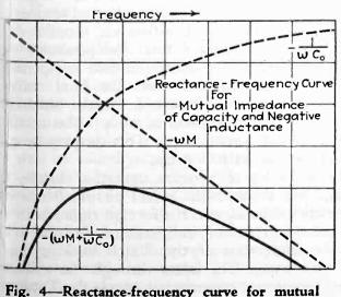
Fig. 4—Reactance-frequency curve for mutual impedance of capacity and negative inductance
