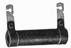
ture-proof enamel. Contact bands and soldering lugs are of Monel metal. The lugs are solder-dipped for easy connection. All parts expand equally under load. The overall length of the unit is 2 inches, with a maximum outside diameter of  $\frac{5}{8}$  inches. It is made with resistance ratings from 10,000 to 250,-000 ohms.—*Electronics, Sept., 1930.*
