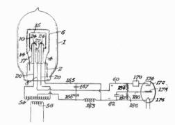
Rectifier and voltage regulator. Two patents granted to T. E. Foulke and assigned to General Electric Vapor Lamp Company, Hoboken, N. J., dealing with a combination of a gaseous rectifier and a voltage regulator in a single envelope. Nos. 1,772,562 and 1,772,603.
