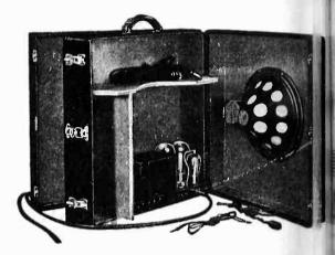
Amplifier unit designed by QRS-DeVr Corporation, Chicago. One 224, one 25 and one 281 tube are used. The speake section may be removed from the case
