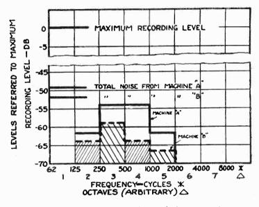
Fig. 5-Annoyance analysis of disc turntable mechanical vibration
