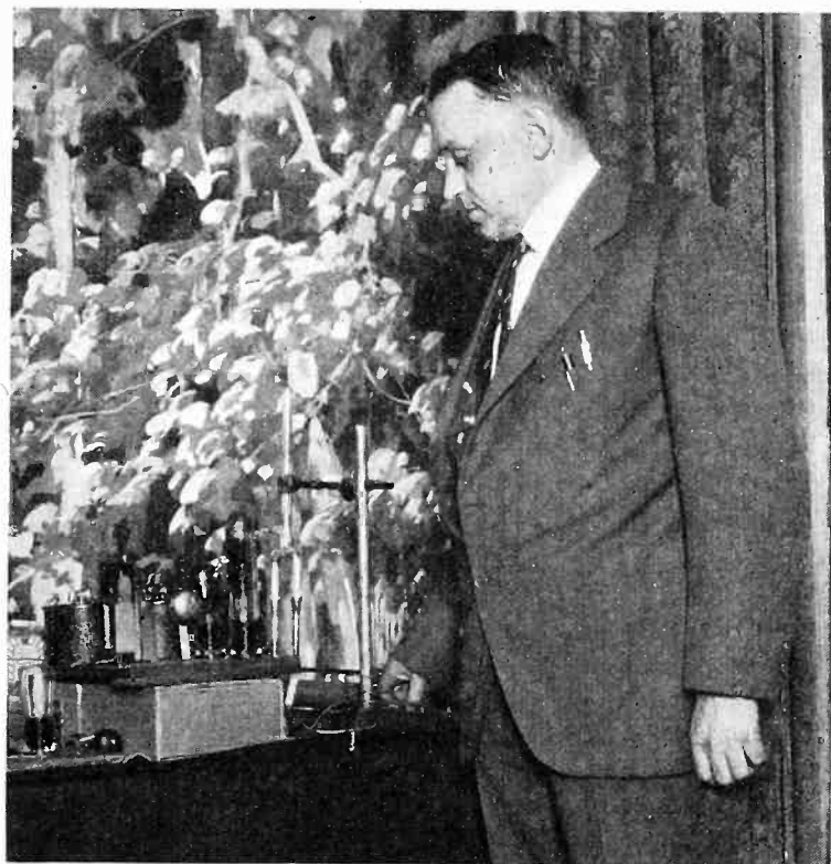
Dr. H. C. Rentschler and his ultra-violet dosage meter. A condenser is permitted to charge by the photo-electric cell so long as radiation falls upon the latter. The condenser discharges at regular intervals and registers the amount of ultra-violet that has fallen on the cell—and on the patient.
