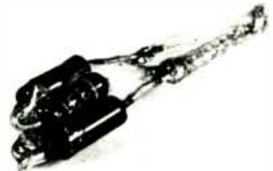
Fig. 4. Solid-state thermometer circuit using a transistor as an amplifying sensor instead of a diode. This circuit requires more stable resistors and power supply than circuit of Fig. 2.
