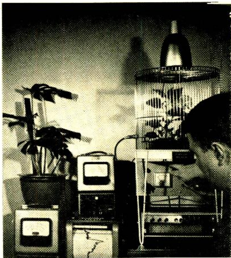
Fig. 4. Experimental setup using Backster Effect for checking psi phenomena in living plants by subjecting them to artificial excitations (currents, red light, etc.), and monitoring responses. Note the red-light growth stimulator on Faraday cage.
