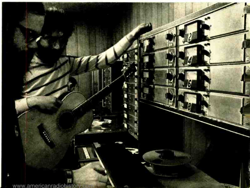
Author and guitarist Jerry Garcia listen to one of sixteen available tracks recorded on the multitrack recorder/reproducer, following a recording session of the "Grateful Dead." The recorder allows Garcia and other members of the group to record individually, and at different times, and later the tracks are mixed for the master tape. This technique permits a wide variety of special effects which identify the group.
