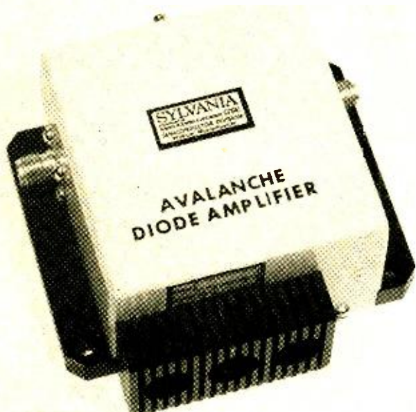
Fig. 3. Three-stage avalanche-diode amplifier package.
