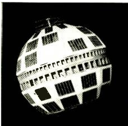
Telstar, launched July 10, 1962, was the second medium-altitude comsat to use active repeater. Developed by Bell System and launched by NASA, the 175-lb satellite provided the first transatlantic TV and telephone transmissions. Spiral antenna at top was for telemetry and command, while communications signals were handled by phased array around the middle.
