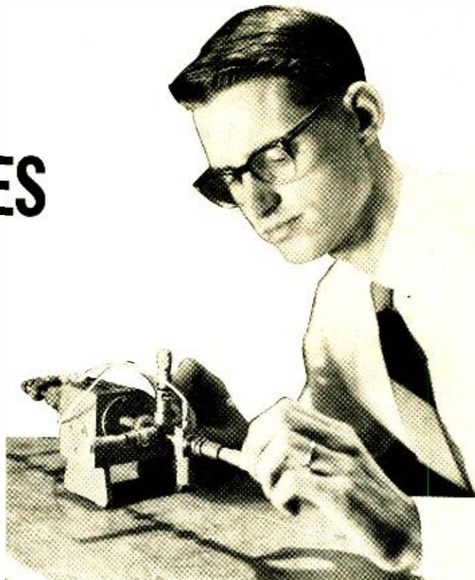
Dr. John A. Copeland adjusts an experimental solid-state millimeter oscillator which replaces cumbersome klystron.
