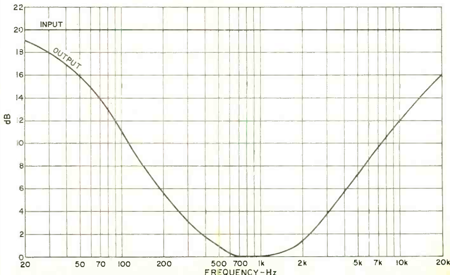
Fig. 2. Measured performance of the circuit of Fig. 1. Since this circuit has no voltage gain, higher amplifier gain settings are required to maintain volume at its previous levels.
