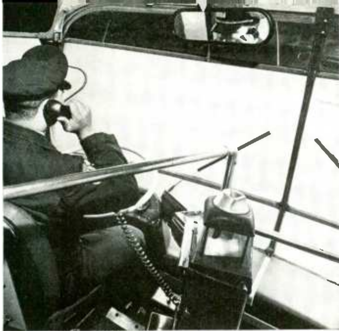
New York City bus driver is using his handset to communicate by two-way radio with his headquarters dispatcher. Hidden behind driver is a gooseneck-mounted mike for bus p.a. system.
