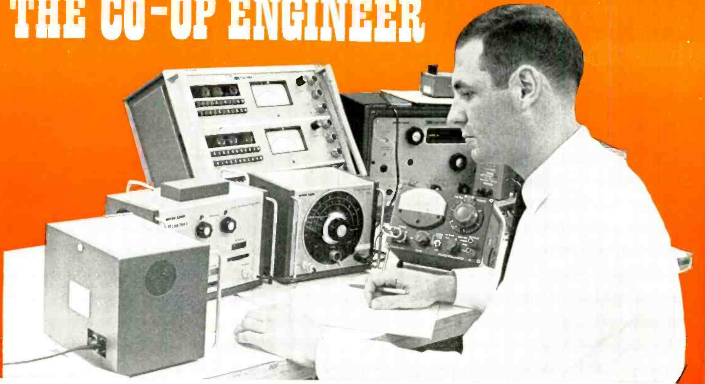
The co-op engineer uses many kinds of test equipment. Here the student is making measurements with Wayne-Kerr bridge.
