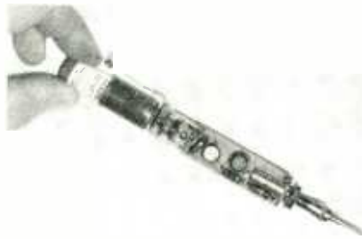
Fig. 2. Components are mounted on a phenolic board and then slipped into a plastic tube of 3/4" Bakelite. Refer to text.
